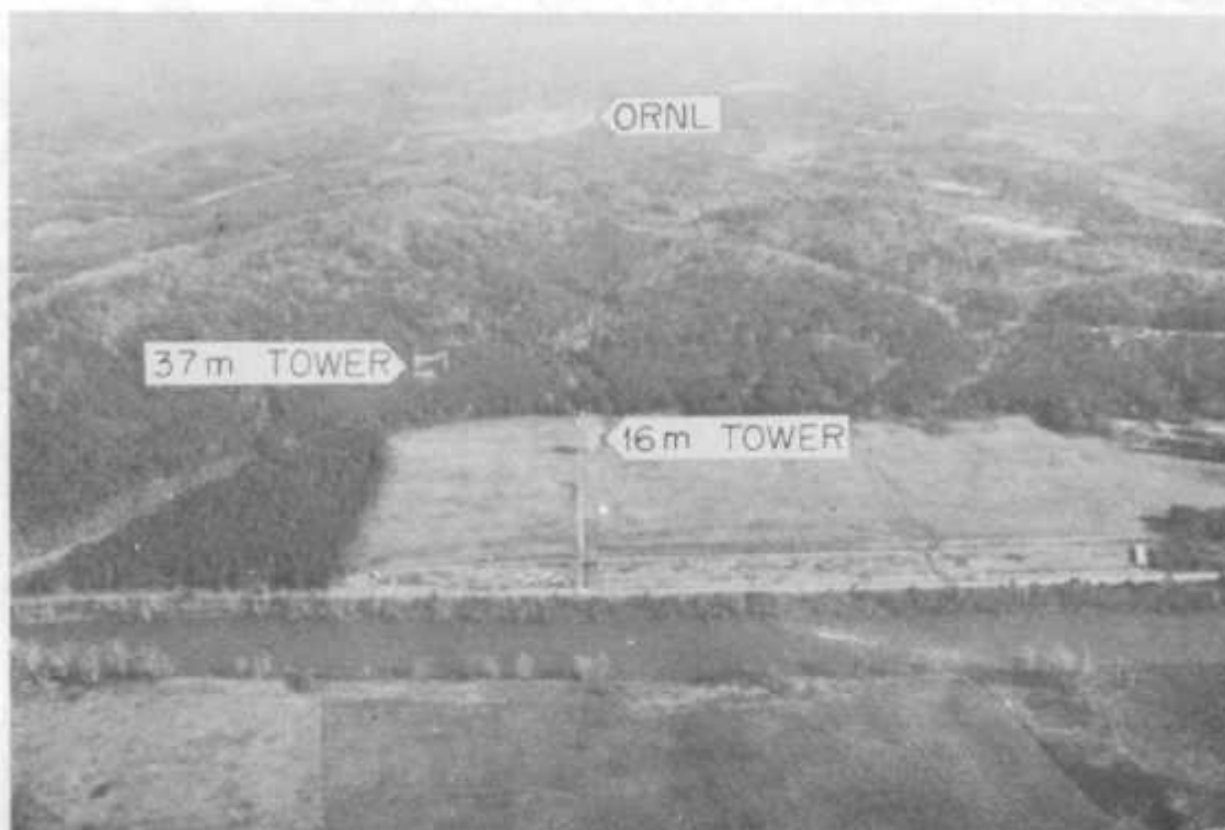
Fig.1. Aerial view, looking north-northeast, of pine plantation and surroundings. Instrumented 37 m forest tower is visible to left of center. Strong winds are most often from southwest. Smoke is being emitted from both towers in this photo.
