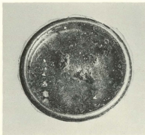
Figure 21. Ashes from a sheet of sticky paper sealed with tape in a 1-in.-diameter planchet.
