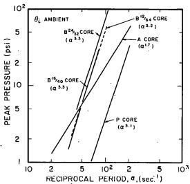
Fig. 145 Peak transient pressure for Spert I cores as a function of reciprocal reactor period.
