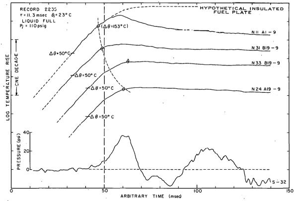
Fig. 50 A presentation of fuel-plate surface temperature-time histories at various radial positions and the pressure-time history for a specific initial pressure with the reactor vessel liquid full. The symbol  $\theta$  on the temperature-time histories indicates the boiling temperature with the corresponding temperature rise shown in parentheses adjacent to one of the traces.
