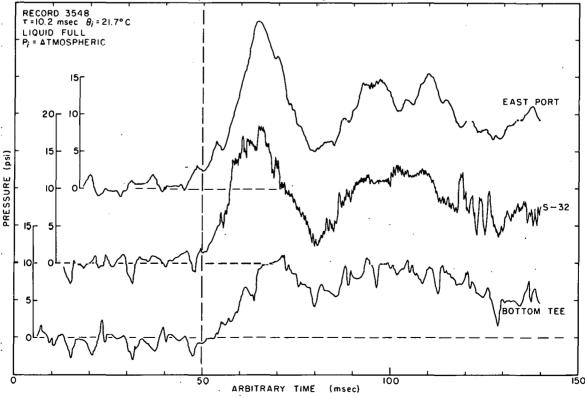
Fig. 65 Representative pressure-time histories for various locations in the Spert III reactor vessel and atmospheric initial system pressure.
