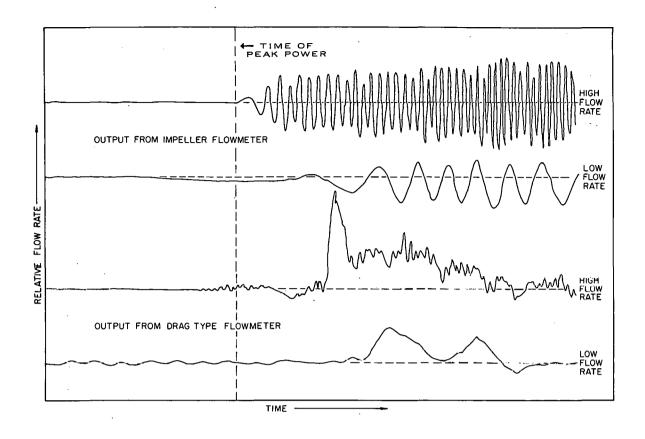
Fig. 4 Typical outputs from impeller and drag-type flowmeters for high and low flow rates.
