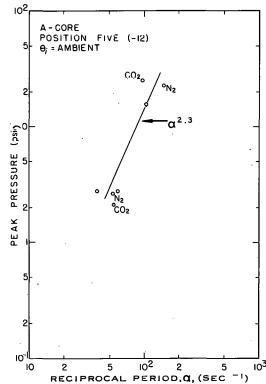
Fig. 99 Peak transient pressure at long-itudinal position 5 inside an A-Core fuel assembly as a function of reciprocal reactor period.
