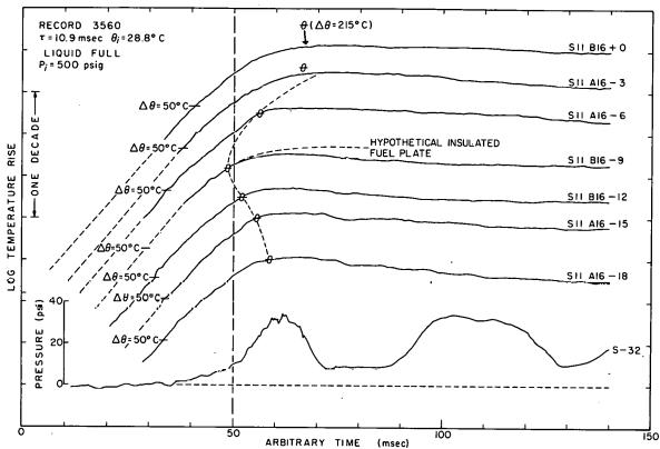
Fig. 53 A presentation of fuel-plate surface temperature-time histories at various longitudinal positions along a fuel plate and the pressure-time history for a specific initial pressure with the reactor vessel liquid full. The symbol  $\theta$  on the temperature-time histories indicates the boiling temperature with the corresponding temperature rise shown in parentheses adjacent to one of the traces.
