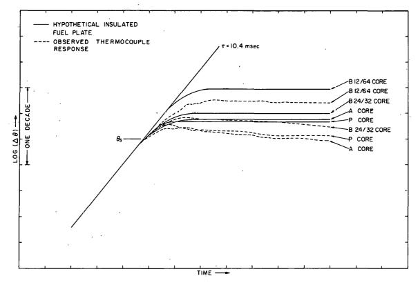
Fig. 147 Representative temperature-time histories and hypothetical insulated-plate behaviors for the Spert I cores.
