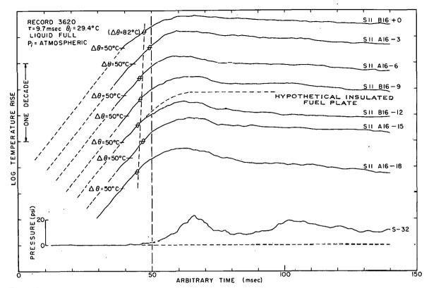
Fig. 49 A presentation of fuel-plate surface temperature-time histories at various longitudinal positions along a fuel plate and the pressure-time history. The symbol  $\theta$  on the temperature-time histories indicates the boiling temperature with the corresponding temperature rise shown in parentheses adjacent to one of the traces.
