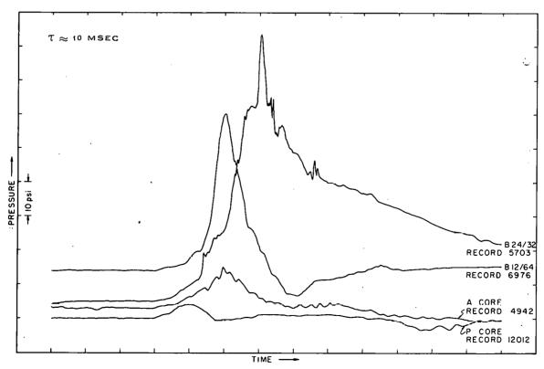
Fig. 144 Representative pressure-time histories for Spert I Cores, time normalized at first perceptible deflection of pressure-time histories.
