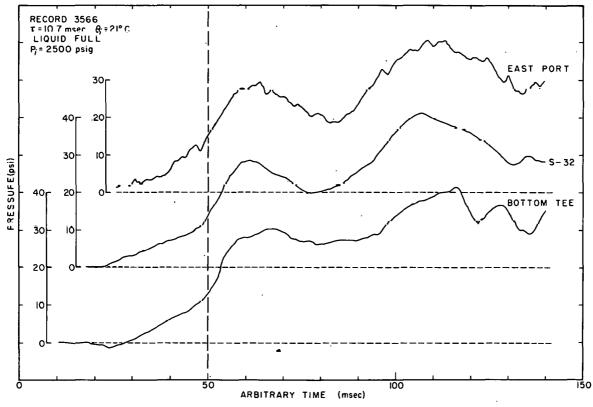
Fig. 67 Representative pressure-time histories for various locations in the Spert III reactor vessel and 2500 psig initial system pressure.
