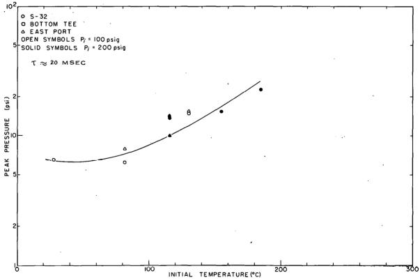
Fig. 76 Peak transient pressure as a function of initial system temperature for a liquid full reactor vessel and various initial system pressures.
