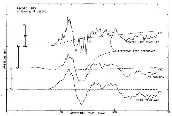
Fig. 29 Representative pressure-time histories obtained at various locations within the reactor tank for a nominal 13-msec reactor period.
