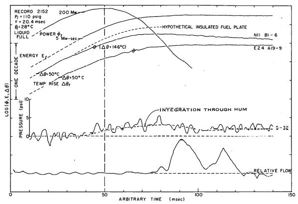
Fig. 58 A presentation of time histories for power, energy, fuel-plate surface temperature, pressure, and flow for a specific initial pressure with the reactor vessel liquid full. The symbol  $\theta$  on the temperature-time histories indicates the boiling temperature with the corresponding temperature rise shown in parentheses adjacent to one of the traces.
