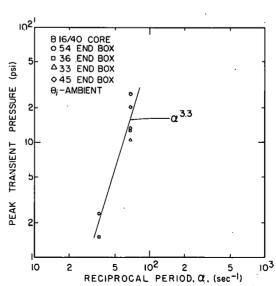
Fig. 135 Peak transient pressure in various lower end boxes of B 16/40 fuel assemblies as a function of reciprocal reactor period.
