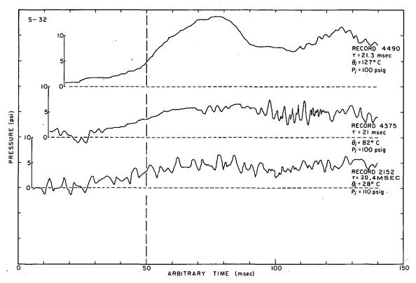
Fig. 60 Representative pressure-time histories for various initial system temperatures.
