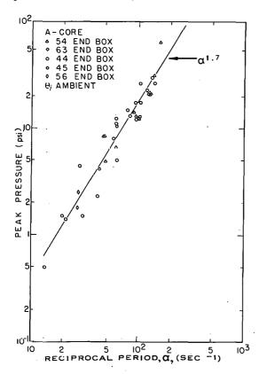
Fig. 103 Peak transient pressure in various lower end boxes as a function of reciprocal reactor period with pure water moderator.
