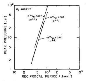
Fig. 137 Peak transient pressure as measured in the lower endboxes of fuel assemblies in the three B-Cores as a function of reciprocal reactor period.
