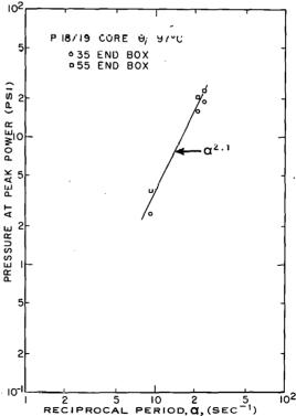
Fig. 36 Transient pressure at time of peak power in various lower end boxes as a function of reciprocal reactor period for boiling initial temperature.
