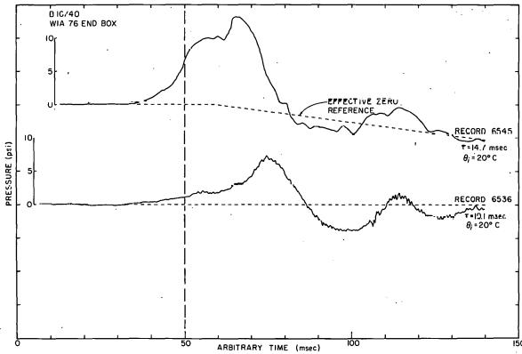
Fig. 124 Representative B 16/40 Core pressure-time histories for ambient temperature reactor transients at various reactor periods.
