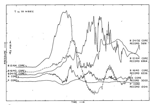
Fig. 143 Representative pressure-time histories for Spert I Cores, time normalized at first perceptible deflection of pressure-time histories.
