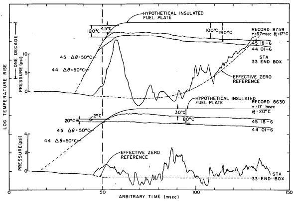
Fig. 24 Representative pressure-time histories for P-Core transients indicating typical deviations from the behavior of a hypothetical insulated fuel plate.
