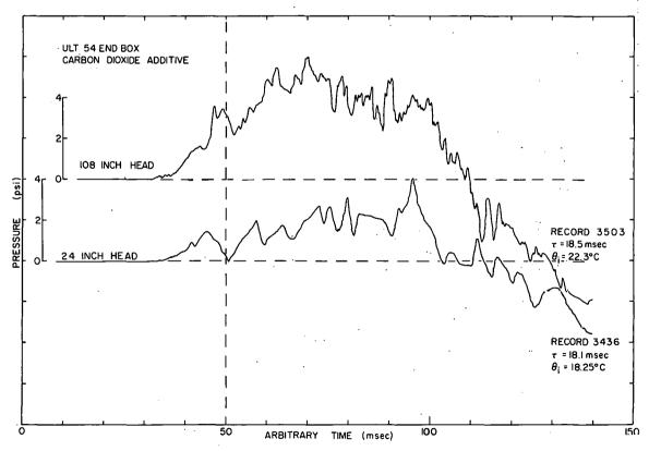
Fig. 91 Representative pressure-time histories for various depths of water head above the reactor core with carbon dioxide additive in the moderator.
