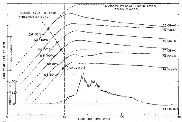
Fig. 113 A presentation of fuel-plate surface temperature-time histories at various radial positions and the pressure-time history. The symbol  $\theta$  on the temperature-time histories indicates the boiling temperature with the corresponding temperature rise shown in parentheses adjacent to one of the traces.
