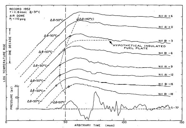
Fig. 56 A presentation of fuel-plate surface temperature-time histories at various longitudinal positions along a fuel plate and the pressure-time history for a specific initial pressure with an air dome in the reactor vessel. The symbol  $\theta$  on the temperature-time histories indicates the boiling temperature with the corresponding temperature rise shown in parentheses adjacent to one of the traces.
