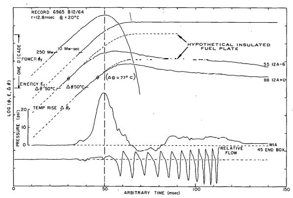
Fig. 110 A presentation of time histories for power, energy, fuel-plate surface temperature, pressure, and flow. The symbol  $\theta$  on the temperature-time histories indicates the boiling temperature with the corresponding temperature rise shown in parentheses adjacent to one of the traces.
