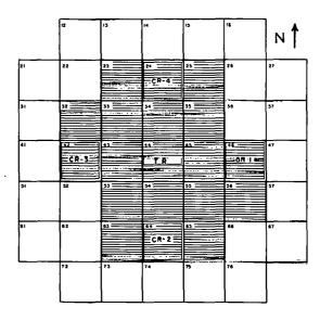
Fig. 11 Layout of Sport I reactor grid showing arrangement of fuel assemblies for the operational P-Core.
