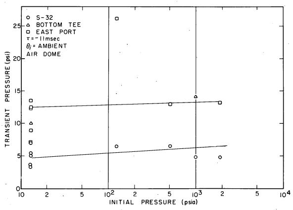
Fig. 71 Peak transient pressure as a function of initial system pressure for ambient initial temperature reactor transients, conducted with an air dome in the reactor vessel.
