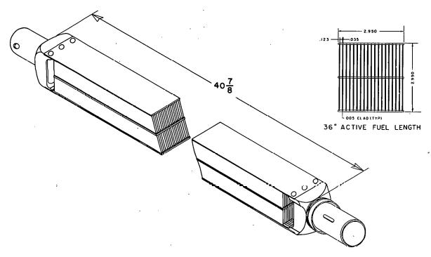
Fig. 41 Schematic representation of a standard, stainless steel, Spert III fuel assembly.
