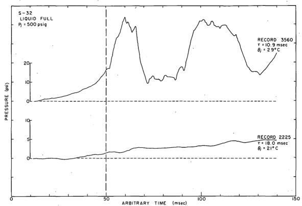
Fig. 64 Representative pressure-time histories for various reactor periods and 500 psig initial system pressure.
