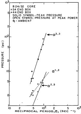
Fig. 134 Peak transient pressure and transient pressure at time of peak power in various lower end boxes of B 24/32 fuel assemblies as a function of reciprocal reactor period.
