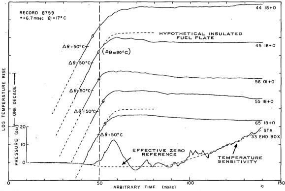
Fig. 22 A presentation of fuel-plate surface temperature-time histories at various radial positions and the pressure-time history. The symbol  $\theta$  on the temperature-time histories indicates the boiling temperature with the corresponding temperature rise shown in parentheses adjacent to one of the traces.
