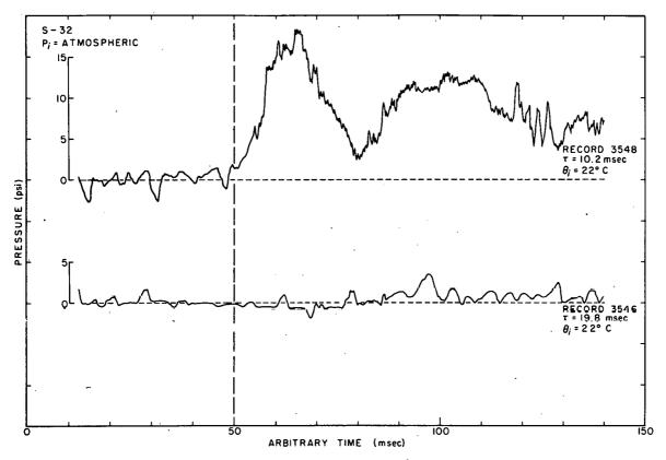
Fig. 62 Representative pressure-time histories for various reactor periods and atmospheric initial system pressure.
