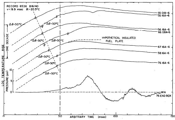
Fig. 115 A presentation of fuel-plate surface temperature-time histories at various radial positions and the pressure-time history. The symbol  $\theta$  on the temperature-time histories indicates the boiling temperature with the corresponding temperature rise shown in parentheses adjacent to one of the traces.
