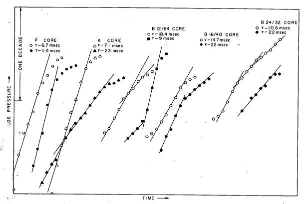
Fig. 142 Display of the degree of fit obtained when exponential functions are normalized to the Spert I pressure-time histories.
