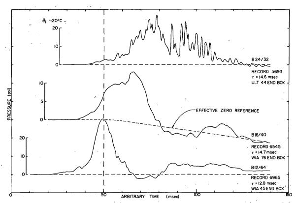
Fig. 129 Representative pressure-time histories for the three B-Cores at ambient initial temperature.
