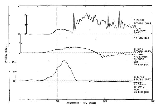
Fig. 131 Representative pressure-time histories for the three B-Cores at a nominal 60°C initial temperature.
