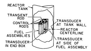
Fig. 28 Schematic representation of transducer locations for investigation of directional aspects of pressure generation.
