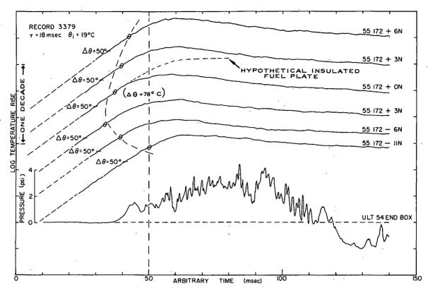
Fig. 83 A presentation of fuel-plate surface temperature-time histories at various longitudinal positions along a fuel plate and the pressure-time history. The symbol  $\theta$  on the temperature-time histories indicates the boiling temperature with the corresponding temperature rise shown in parentheses adjacent to one of the traces.
