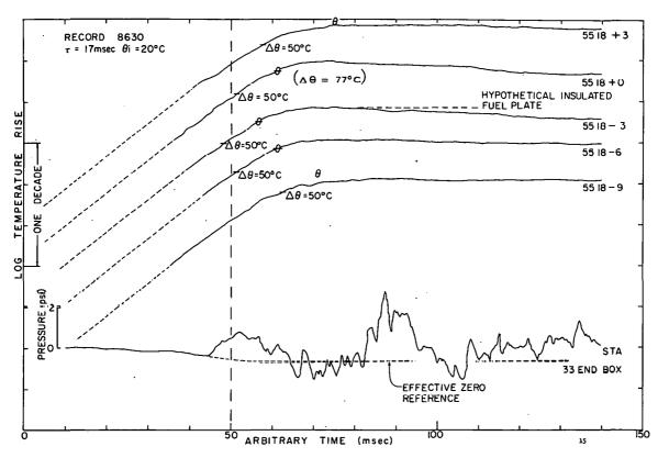
Fig. 19 A presentation of fuel-plate surface temperature-time histories at various longitudinal positions along a fuel plate and the pressure-time history. The symbol  $\theta$  on the temperature-time histories indicates the boiling temperature with the corresponding temperature rise shown in parentheses adjacent to one of the traces.
