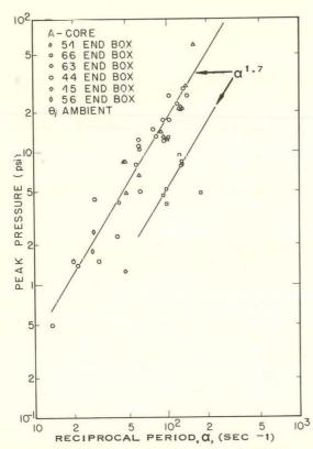
Fig. 96 Peak transient pressure in various lower end boxes as a function of reciprocal reactor period.
