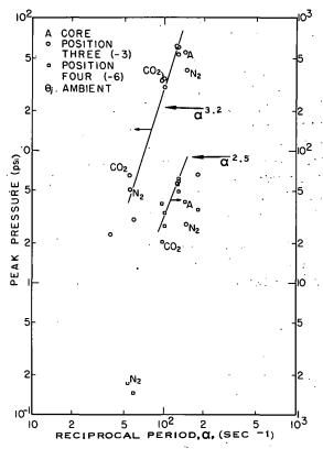
Fig. 98 Peak transient pressure at longitudinal positions 3 and 4 inside an A-Core fuel assembly as a function of reciprocal reactor period.
