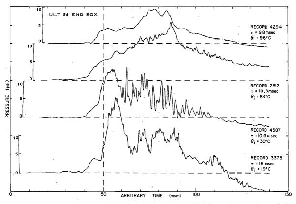
Fig. 89 Representative pressure-time histories for various initial temperatures and a nominal 10-msec reactor period.
