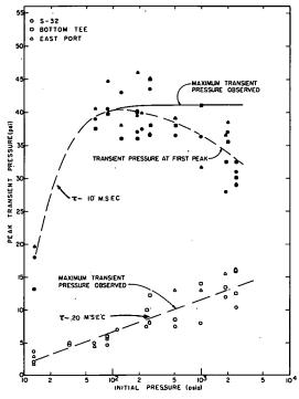
Fig. 70 Peak transient pressure as a function of initial system pressure for ambient initial temperature reactor transients, conducted with the reactor vessel liquid full.
