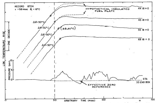
Fig. 20 A presentation of fuel-plate surface temperature-time histories at various radial positions and the pressure-time history. The symbol  $\theta$  on the temperature-time histories indicates the boiling temperature with the corresponding temperature rise shown in parentheses adjacent to one of the traces.
