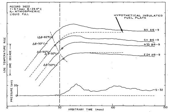
Fig. 48 A presentation of fuel-plate surface temperature-time histories at various radial positions and the pressure-time history. The symbol  $\theta$  on the temperature-time histories indicates the boiling temperature with the corresponding temperature rise shown in parentheses adjacent to one of the traces.
