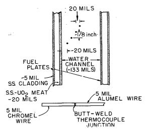
Fig. 15 Schematic representation of the placement of thermocouples for temperature measurements obtained between fuel plates in the Spert 1 P-Core fuel assembly.
