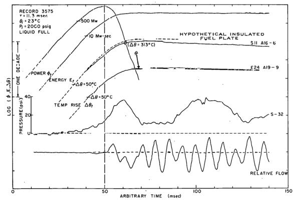
Fig. 47. A presentation of time histories for power, energy, fuel-plate surface temperature, pressure, and flow for a specific initial pressure with the reactor vessel liquid full. The symbol  $\theta$  on the temperature-time histories indicates the boiling temperature with the corresponding temperature rise shown in parentheses adjacent to one of the traces.
