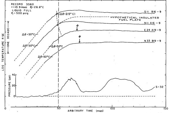
Fig. 52 A presentation of fuel-plate surface temperature-time histories at various radial positions and the pressure-time history for a specific initial pressure with the reactor vessel liquid full. The symbol  $\theta$  on the temperature-time histories indicates the boiling temperature with the corresponding temperature rise shown in parentheses adjacent to one of the traces.
