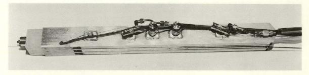
Fig. 94  $\,$  Photograph of a special Spert I A-Core fuel assembly with pressure transducers mounted in a side plate and in the lower end box.
