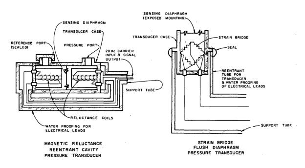
Fig. 5 Schematic representation of pressure transducers showing the flush diaphragm and reentrant cavity designs.
