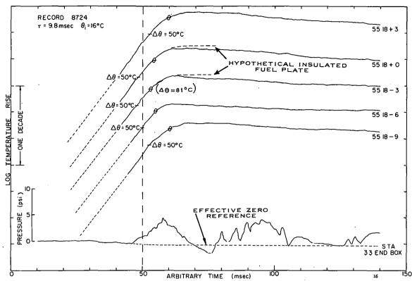
Fig. 21 A presentation of fuel-plate surface temperature-time histories at various longitudinal positions along a fuel plate and the pressure-time history. The symbol  $\theta$  on the temperature-time histories indicates the boiling temperature with the corresponding temperature rise shown in parentheses adjacent to one of the traces.
