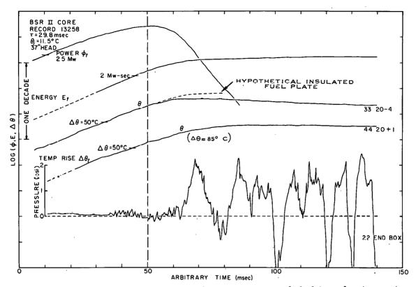
Fig. 139 A presentation of time histories for power, energy, fuel-plate surface temperature, pressure, and flow. The symbol  $\theta$  on the temperature-time histories indicates the boiling temperature with the corresponding temperature rise shown in parentheses adjacent to one of the traces.
