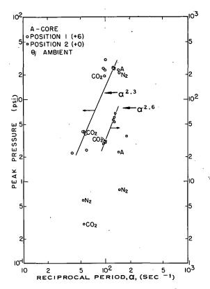
Fig. 97 Peak transient pressure at longitudinal positions 1 and 2 inside an A-Core fuel assembly as a function of reciprocal reactor period.
