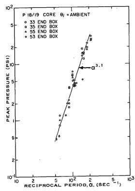
Fig. 33 Peak transient pressure in various lower end boxes as a function of reciprocal reactor period for ambient initial temperature.
