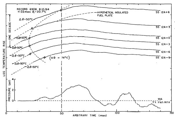
Fig. 120 A presentation of fuel-plate surface temperature-time histories at various longitudinal positions along a fuel plate and the pressure-time history. The symbol  $\theta$  on the temperature-time histories indicates the boiling temperature with the corresponding, temperature rise shown in parentheses adjacent to one of the traces.
