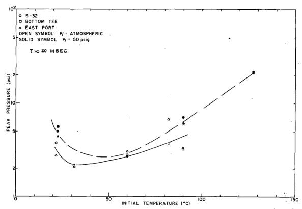
Fig. 75 Peak transient pressure as a function of initial system temperature for a liquid full reactor vessel and various initial system pressures.
