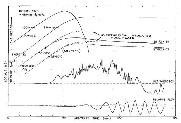
Fig. 80 A presentation of time histories for power, energy, fuel-plate surface temperature, pressure, and flow. The symbol  $\theta$  on the temperature-time histories indicates the boiling temperature with the corresponding temperature rise shown in parentheses adjacent to one of the traces.
