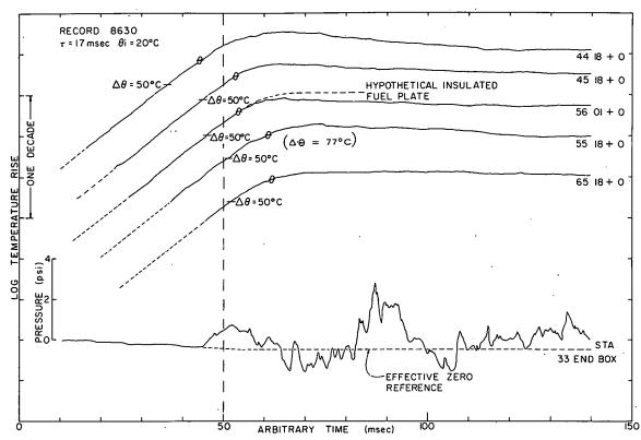
Fig. 17 A presentation of fuel-plate surface temperature-time histories at various radial positions and the pressure-time history. The symbol  $\theta$  on the temperature-time histories indicates the boiling temperature with the corresponding temperature rise shown in parentheses adjacent to one of the traces.
