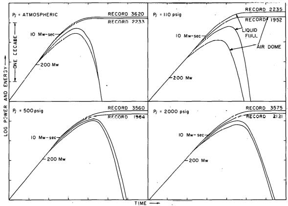
Fig. 57 Representative power and energy-time histories for reactor transients conducted with the reactor vessel liquid full and with an air dome in the vessel.
