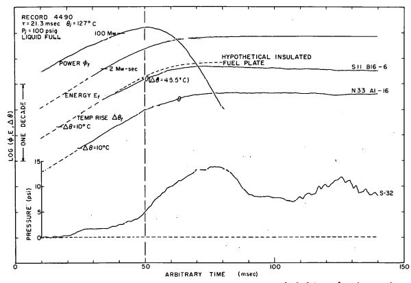
Fig. 59 A presentation of time histories for power, energy, fuel plate surface temperature, and pressure, for a specific initial pressure with the reactor vessel liquid full. The symbol  $\theta$  on the temperature-time histories indicates the boiling temperature with the corresponding temperature rise shown in parentheses adjacent to one of the traces.
