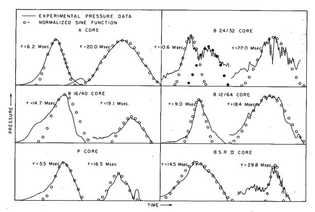
Fig. 141 Display of the degree of fit obtained when sine functions are normalized to the Spert I pressure-time histories.
