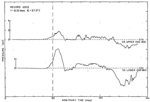
Fig. 32 Pressure-time histories obtained in upper and lower end boxes of a P-Core fuel assembly.
