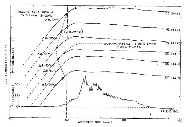
Fig. 114 A presentation of fuel-plate surface temperature-time histories at various longitudinal positions along a fuel plate and the pressure-time history. The symbol  $\theta$  on the temperature-time histories indicates the boiling temperature with the corresponding temperature rise shown in parentheses adjacent to one of the traces.
