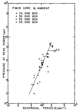
Fig. 34 Transient pressure at time of peak power in various lower end boxes as a function of reciprocal reactor period for ambient initial temperature.
