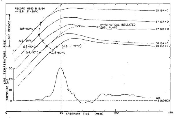
Fig. 121 A presentation of fuel-plate surface temperature-time histories at various radial positions and the pressure-time history. The symbol  $\theta$  on the temperature-time histories indicates the boiling temperature with the corresponding temperature rise shown in parentheses adjacent to one of the traces.
