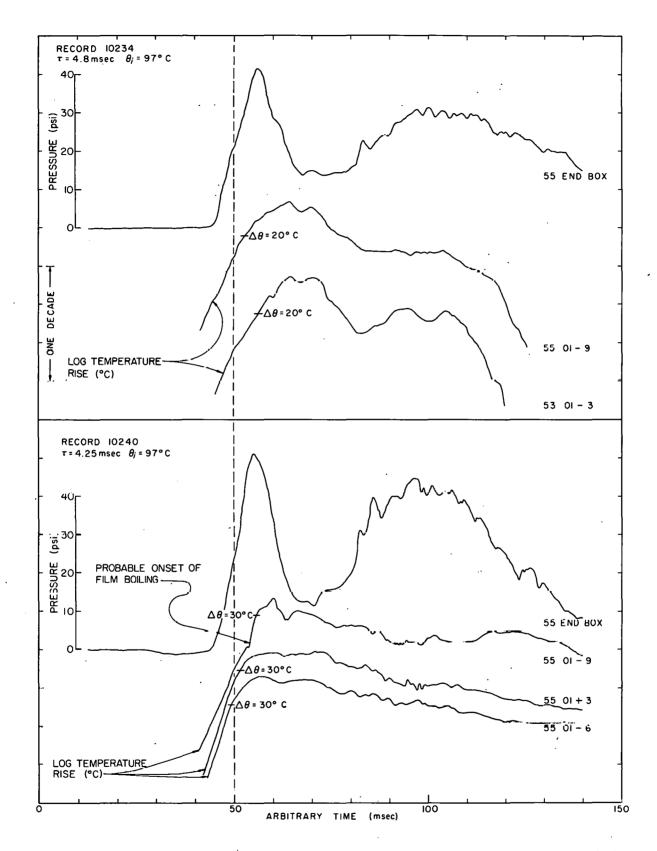
Fig. 25 Representative temperature- and pressure-time histories for boiling reactor transients showing correlations between the occurrence of heat transfer from the fuel plate to the moderator water and the resultant pressure generation.
