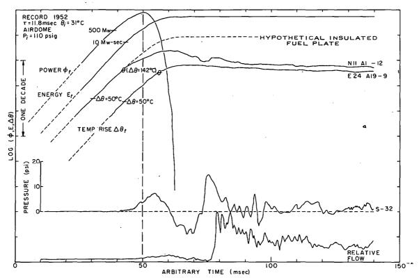
Fig. 54 A presentation of time histories for power, energy, fuel-plate surface temperature, pressure, and flow for a specific initial pressure with an air dome in the reactor vessel. The symbol  $\theta$  on the temperature-time histories indicates the boiling temperature with the corresponding temperature rise shown in parentheses adjacent to one of the traces.
