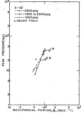
Fig. 74 Peak transient pressure as a function of reciprocal reactor period for ambient initial temperature reactor transients and various initial system pressures.
