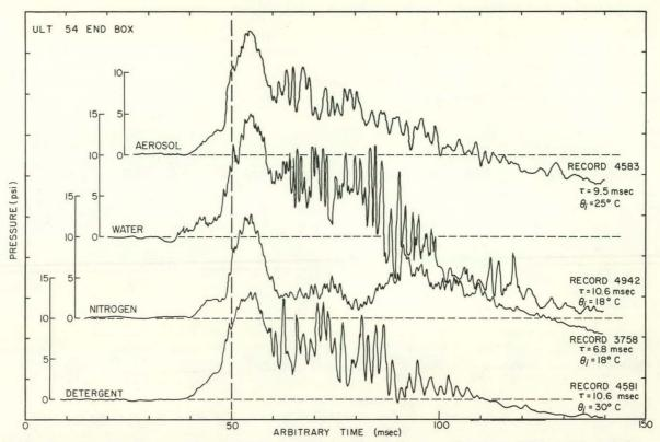
Fig. 93 Representative pressure-time histories with various moderator additives present for a nominal 10-msec reactor period.
