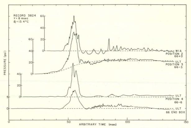
Fig. 95 Representative pressure-time histories obtained inside a special Spert I fuel assembly.
