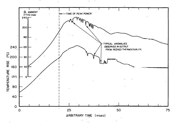
Fig. 2 Anomalous temperature behavior observed with peened thermocouples used in Spert I transient testing.
