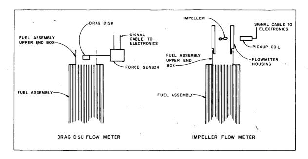
Fig. 3 Schematic representation of impeller and drag disc flowmeters used in Spert transient testing.
