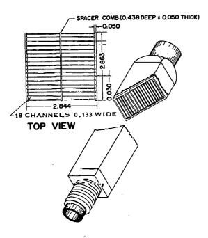
Fig. 10 Schematic representation of stainless steel P-Core fuel assembly.
