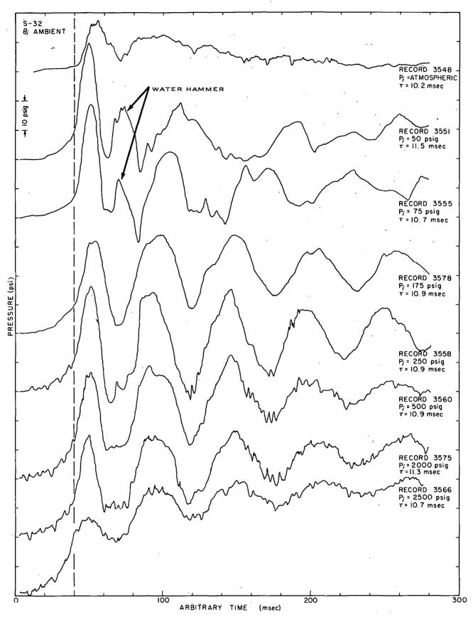
Fig. 68 Representative pressure-time histories for reactor transients conducted at various initial system pressures.
