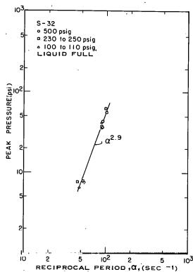
Fig. 73 Peak transient pressure as a function of reciprocal reactor period for ambient initial temperature reactor transients and various initial system pressures.
