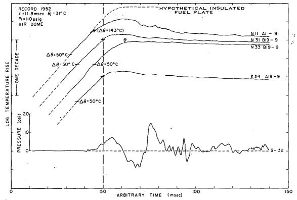
Fig. 55 A presentation of fuel-plate surface temperature-time histories at various radial positions and the pressure-time history for a specific initial pressure with an air dome in the reactor vessel. The symbol  $\theta$  on the temperature-time histories indicates the boiling temperature with the corresponding temperature rise shown in parentheses adjacent to one of the traces.
