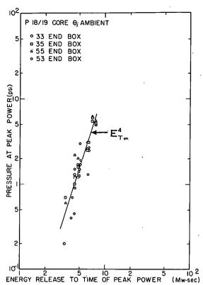
Fig. 38 Transient pressure at time of peak power in various lower end boxes as a function of nuclear energy release to time of peak power for ambient initial temperature.
