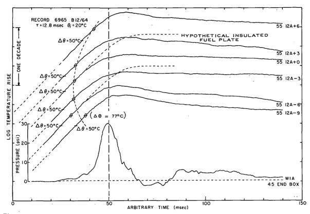
Fig. 122 A presentation of fuel-plate surface temperature-time histories at various longitudinal positions along a fuel plate and the pressure-time history. The symbol  $\theta$  on the temperature-time histories indicates the boiling temperature with the corresponding temperature rise shown in parentheses adjacent to one of the traces.
