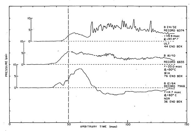
Fig. 132 Representative pressure-time histories for the three B-Cores at a nominal 80°C initial temperature.
