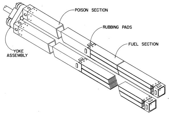
Fig. 42 Schematic representation of a Spert III fuel-poison control rod assembly.
