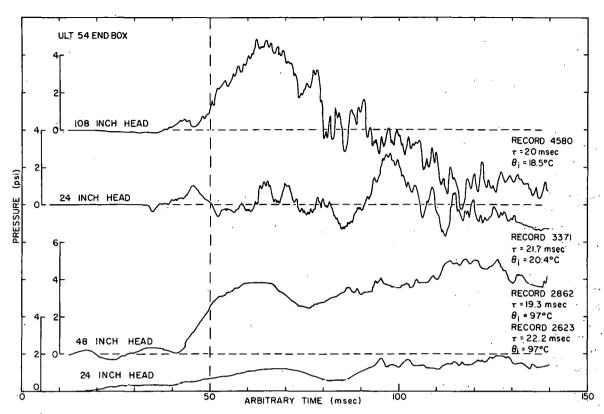
Fig. 90 Representative pressure-time histories for various depths of water head above the reactor core with pure water moderator.
