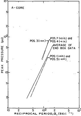
Fig. 100 Peak transient pressure inside an A-Core fuel assembly and in a lower end box as a function of reciprocal reactor period,
