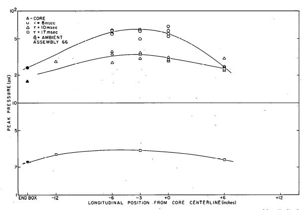
Fig. 101 Peak transient pressure inside an A-Core fuel assembly as a function of longitudinal position in the assembly with pure water moderator.
