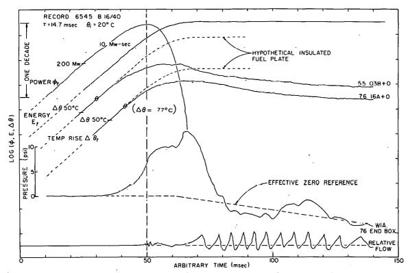
Fig. 109 A presentation of time histories for power, energy, fuel-plate surface temperature, pressure, and flow. The symbol  $\theta$  on the temperature-time histories indicates the boiling temperature with the corresponding temperature rise shown in parentheses adjacent to one of the traces.
