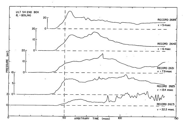
Fig. 87 Representative pressure-time histories for boiling reactor transients at various reactor periods.
