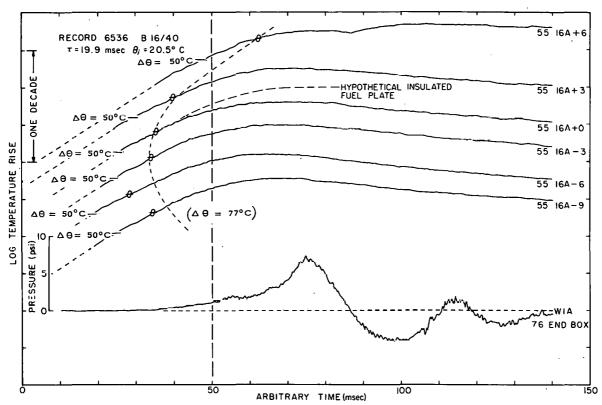
Fig. 116 A presentation of fuel-plate surface temperature-time histories at various longitudinal positions along a fuel plate and the pressure-time history. The symbol  $\theta$  on the temperature-time histories indicates the boiling temperature with the corresponding temperature rise shown in parentheses adjacent to one of the traces.
