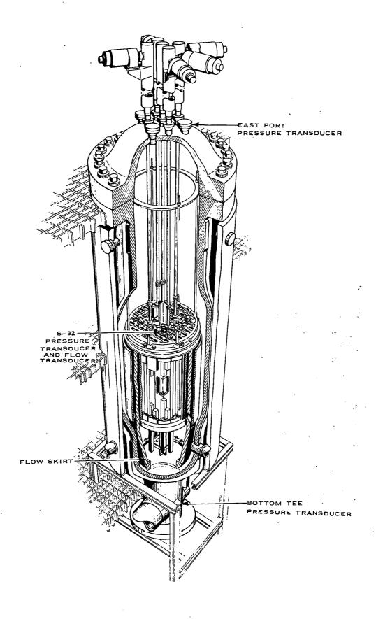
Fig. 40 Schematic representation of Spert III Reactor vessel assembly showing the location of pressure transducers.
