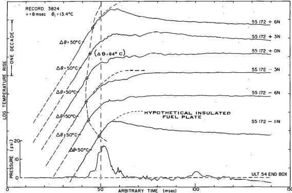
Fig. 84 A presentation of fuel-plate surface temperature-time histories at various longitudinal positions along a fuel plate and the pressure-time history. The symbol  $\theta$  on the temperature-time histories indicates the boiling temperature with the corresponding temperature rise shown in parentheses adjacent to one of the traces.
