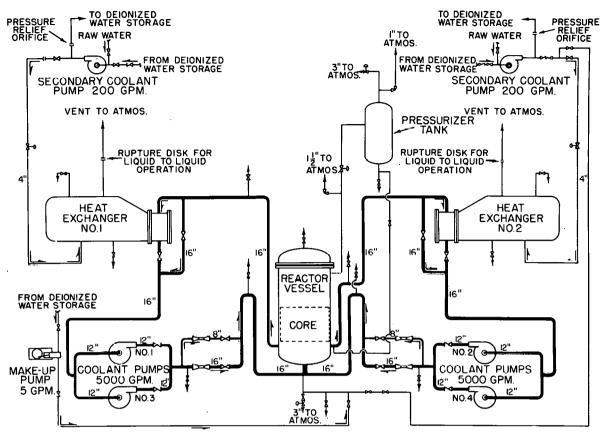
Fig. 39 Schematic representation of Spert III facility showing the reactor vessel and auxiliary equipment.
