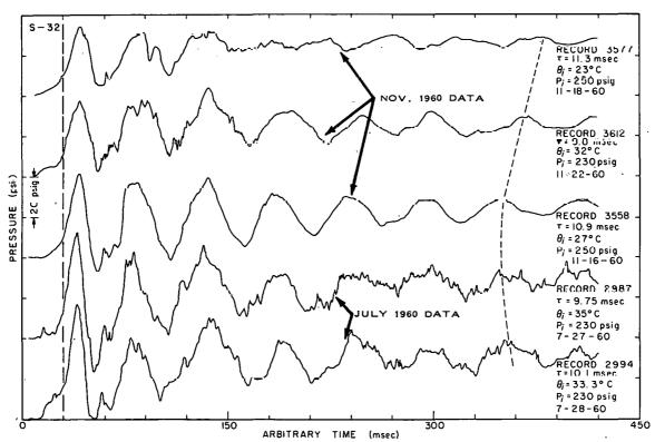
Fig. 69 Representative pressure-time histories showing the degree of repeatability for various transients with similar initial conditions.
