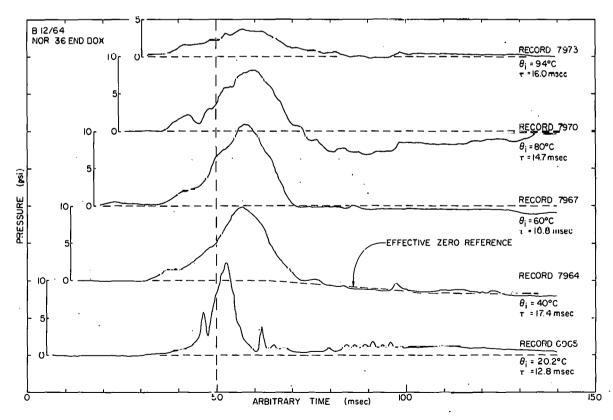
Fig. 128 Representative B 12/64 Core pressure-time histories for various initial temperatures.
