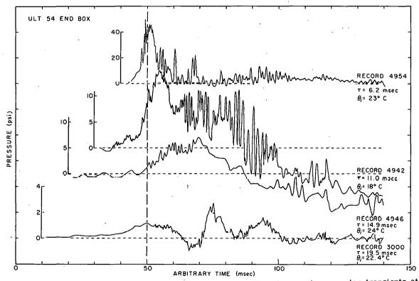
Fig. 86 Representative pressure-time histories for ambient temperature reactor transients at various reactor periods.
