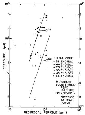
Fig. 136 Peak transient pressure and transient pressure at time of peak power in various lower end boxes of B 12/64 fuel assemblies as a function of reciprocal reactor period.
