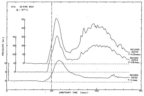
Fig. 27 Representative pressure-time histories for boiling reactor transients showing the dependence upon reactor period.
