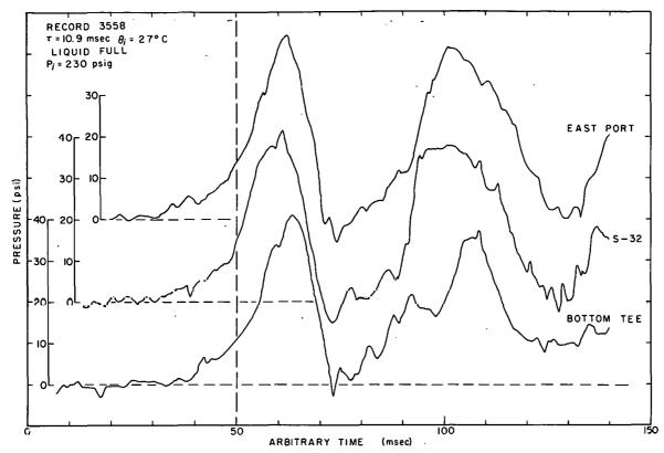
Fig. 66 Representative pressure-time histories for various locations in the Spert III reactor vessel and 230 psig initial system pressure.
