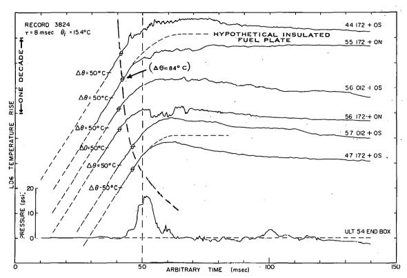
Fig. 85 A presentation of fuel-plate surface temperature-time histories at various radial positions and the pressure-time history. The symbol  $\theta$  on the temperature-time histories indicates the boiling temperature with the corresponding temperature rise shown in parentheses adjacent to one of the traces.
