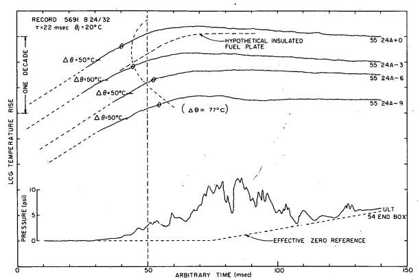
Fig. 112 A presentation of fuel-plate surface temperature-time histories at various longitudinal positions along a fuel plate and the pressure-time history. The symbol  $\theta$  on the temperature-time histories indicates the boiling temperature with the corresponding temperature rise shown in parentheses adjacent to one of the traces.
