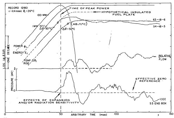
Fig. 13 A presentation of time histories for power, energy, fuel-plate surface temperature, pressure, and flow. The symbol  $\theta$  on the temperature-time histories indicates the boiling temperature with the corresponding temperature rise shown in parentheses adjacent to one of the traces.
