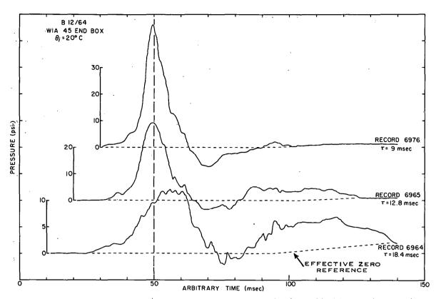
Fig. 125 Representative B 12/64 Core pressure-time histories for ambient temperature reactor transients at various reactor periods.
