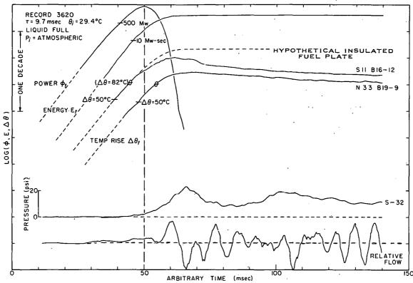
Fig. 44 A presentation of time histories for power, energy, fuel-plate surface temperature, pressure, and flow. The symbol  $\theta$  on the temperature-time histories indicates the boiling temperature with the corresponding temperature rise shown in parentheses adjacent to one of the traces.
