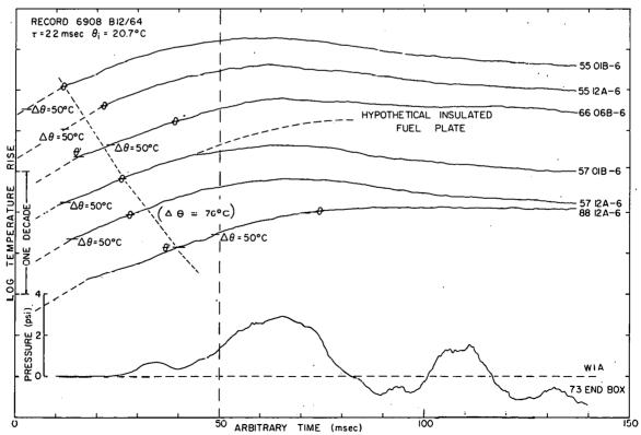
Fig. 119 A presentation of fuel-plate surface temperature-time histories at various radial positions and the pressure-time history. The symbol  $\theta$  on the temperature-time histories indicates the boiling temperature with the corresponding temperature rise shown in parentheses adjacent to one of the traces.
