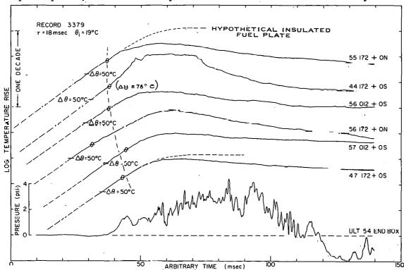
Fig. 82 A presentation of fuel-plate surface temperature-time histories at various radial positions and the pressure-time history. The symbol  $\theta$  on the temperature-time histories indicates the boiling temperature with the corresponding temperature rise shown in parentheses adjacent to one of the traces.
