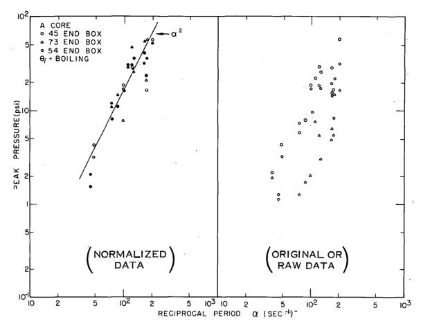
Fig. 105 Raw data and normalized data for peak transient pressures in various lower end boxes during boiling reactor transients.
