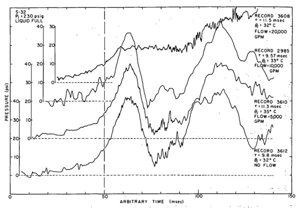
Fig. 61 Representative pressure-time histories for various reactor coolant flow rates.
