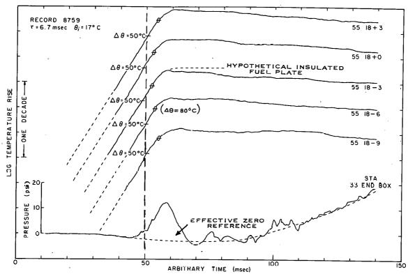
Fig. 23 A presentation of fuel-plate surface temperature-time histories at various longitudinal positions along a fuel plate and the pressure-time history. The symbol  $\theta$  on the temperature-time histories indicates the boiling temperature with the corresponding temperature rise shown in parentheses adjacent to one of the traces.
