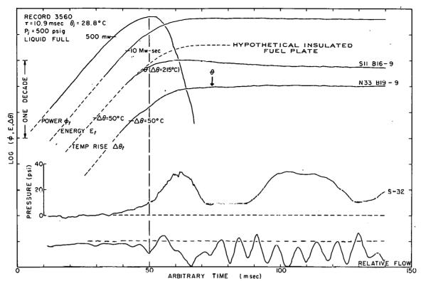
Fig. 46 A presentation of time histories for power, energy, fuel-plate surface temperature, pressure, and flow for a specific initial pressure with the reactor vessel liquid full. The symbol  $\theta$  on the temperature-time histories indicates the boiling temperature with the corresponding temperature rise shown in parentheses adjacent to one of the traces.
