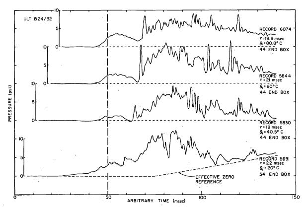
Fig. 126 Representative B 24/32 Core pressure-time histories for various initial temperatures.
