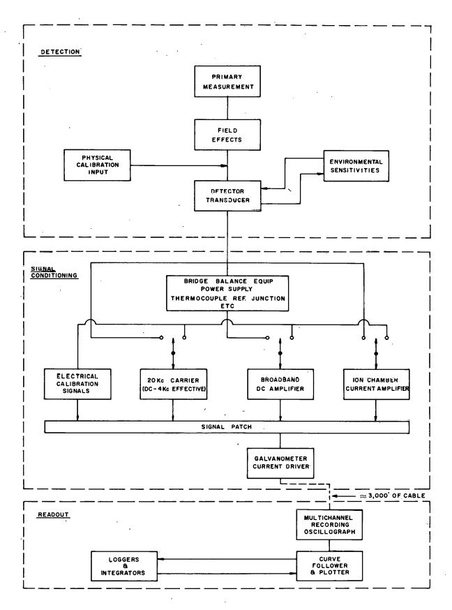
Fig. 1 Schematic representation of the pressure measuring-recording system showing system components and typical problem areas.
