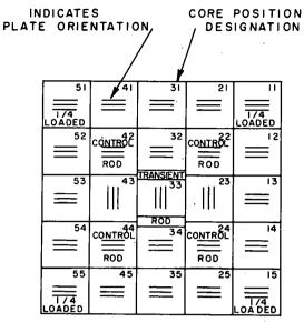
Fig. 138 Layout of Spert I reactor grid showing arrangement of fuel assemblies and fuel-plate orientation for the operational BSR II-Core.
