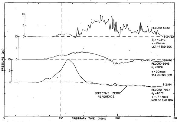
Fig. 130 Representative pressure-time histories for the three B-Cores at a nominal 40°C initial temperature.
