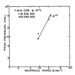
Fig. 35 Peak transient pressure in various lower end boxes as a function of reciprocal reactor period for boiling initial temperature.
