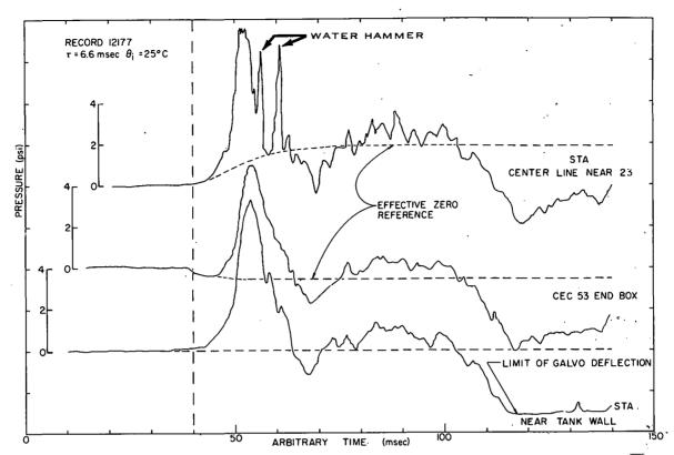
Fig. 30 Representative pressure-time histories obtained at various locations within the reactor tank for a nominal 6.6-msec reactor period.
