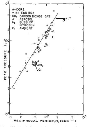
Fig. 104 Peak transient pressure in various lower end boxes as a function of reciprocal reactor period with and without moderator additives.
