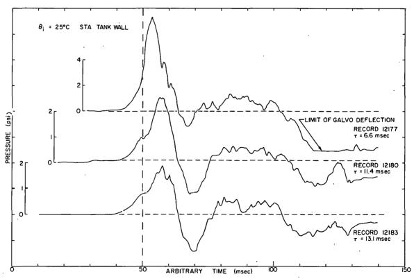
Fig. 31 Pressure-time histories obtained at the wall of the reactor tank for various reactor periods.
