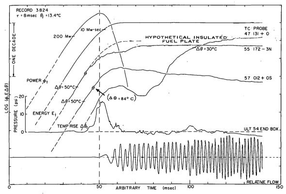
Fig. 81 A presentation of time histories for power, energy, fuel-plate surface temperature, pressure, and flow. The symbol  $\theta$  on the temperature-time histories indicates the boiling temperature with the corresponding temperature rise shown in parentheses adjacent to one of the traces.
