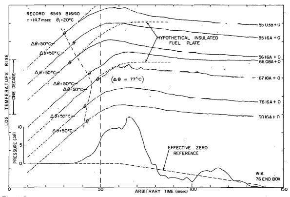
Fig. 117 A presentation of fuel-plate surface temperature-time histories at various radial positions and the pressure-time history. The symbol  $\theta$  on the temperature-time histories indicates the boiling temperature with the corresponding temperature rise shown in parentheses adjacent to one of the traces.
