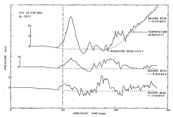
Fig. 26 Representative pressure-time histories for ambient temperature reactor transients showing the dependence upon reactor period. (Note effects of radiation and temperature sensitivity upon the reference pressure level.)
