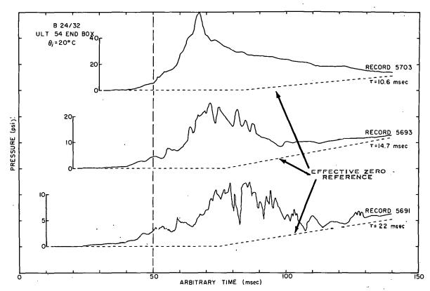
Fig. 123 Representative B 24/32 Core pressure-time histories for ambient temperature reactor transients at various reactor periods.
