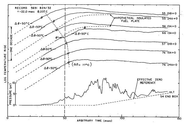
Fig. 111 A presentation of fuel-plate surface temperature-time histories at various radial positions and the pressure-time history. The symbol  $\theta$  on the temperature-time histories indicates the boiling temperature with the corresponding temperature rise shown in parentheses adjacent to one of the traces.
