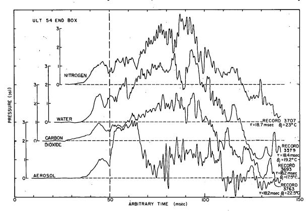
Fig. 92 Representative pressure-time histories with various moderator additives present for a nominal 20-msec reactor period.
