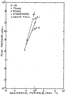
Fig. 72 Peak transient pressure as a function of reciprocal reactor period for ambient initial temperature reactor transients and various initial system pressures.
