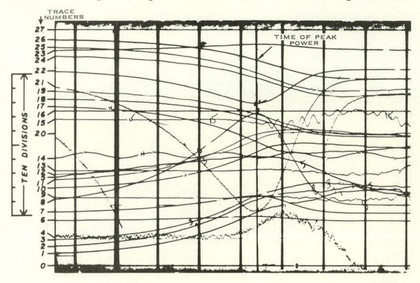
Fig. 12 Photographic reproduction of the original CEC record obtained for a typical Spert I transient.
