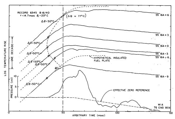
Fig. 118 A presentation of fuel-plate surface temperature-time histories at various longitudinal positions along a fuel plate and the pressure-time history. The symbol  $\theta$  on the temperature-time histories indicates the boiling temperature with the corresponding temperature rise shown in parentheses adjacent to one of the traces.
