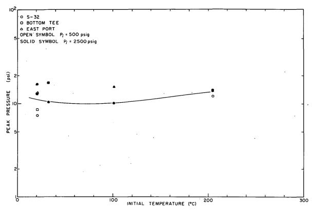
Fig. 77 Peak transient pressure as a function of initial system temperature for a liquid full reactor vessel and various initial system pressures.
