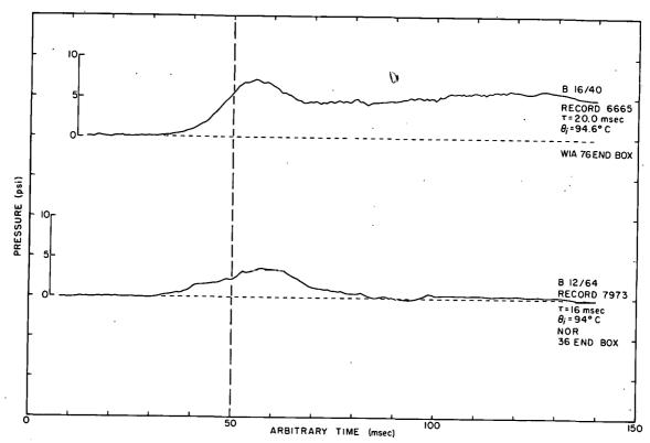
Fig. 133 Representative pressure-time histories for the three B-Cores at a nominal 94°C initial temperature.
