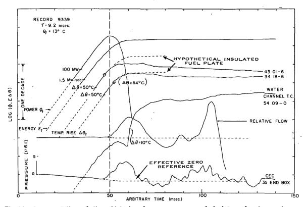
Fig. 14 A presentation of time histories for power, energy, fuel-plate surface temperature, pressure, and flow. The symbol  $\theta$  on the temperature-time histories indicates the boiling temperature with the corresponding temperature rise shown in parentheses adjacent to one of the traces.
