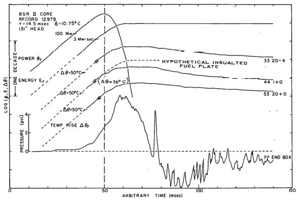
Fig. 140 A presentation of time histories for power, energy, fuel-plate surface temperature, pressure, and flow. The symbol  $\theta$  on the temperature-time histories indicates the boiling temperature with the corresponding temperature rise shown in parentheses adjacent to one of the traces.
