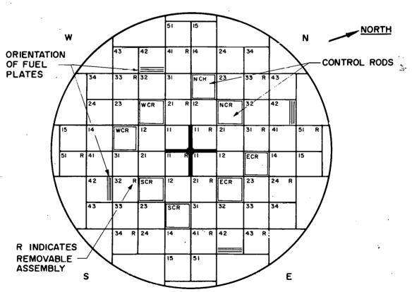
Fig. 43 Layout of Spert III reactor grid showing orientation of fuel plates for a typical fuel assembly in each quadrant.
