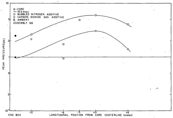
Fig. 102 Peak transient pressure inside an A-Core fuel assembly as a function of longitudinal position in the assembly with moderator additives present.
