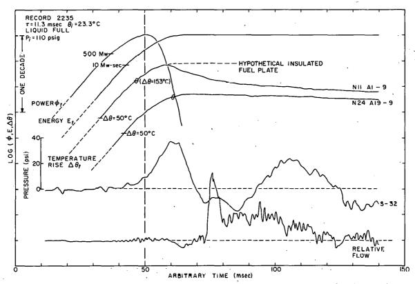
Fig. 45. A presentation of time histories for power, energy, fuel-plate surface temperature, pressure, and flow for a specific initial pressure with the reactor vessel liquid full. The symbol  $\theta$  on the temperature-time histories indicates the boiling temperature with the corresponding temperature rise shown in parentheses adjacent to one of the traces.
