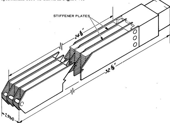
Fig. 78 Schematic representation of aluminum clad A-Core fuel assembly.
