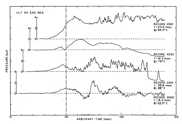
Fig. 88 Representative pressure-time histories for various initial temperatures and a nominal 20-msec reactor period.
