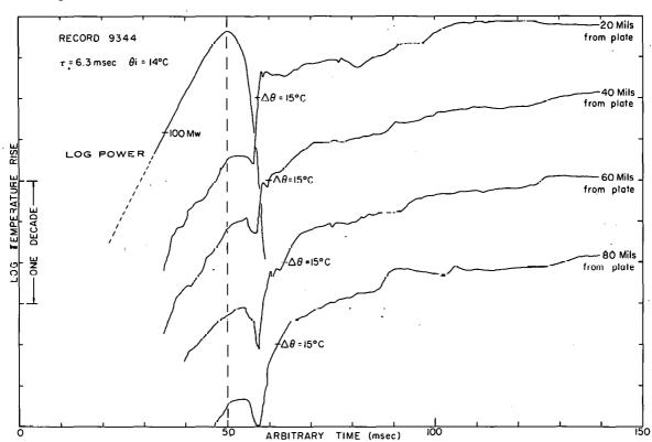
Fig. 16 Temperature-time histories obtained from butt-welded thermocouples in the water channel between fuel plates of the Spert I P-Core assembly.
