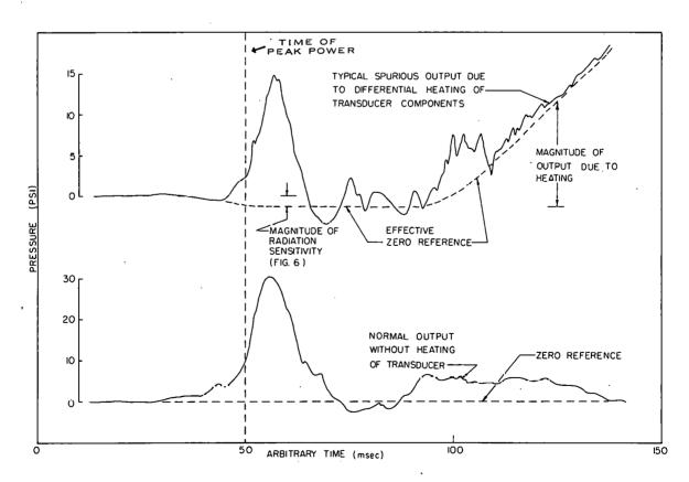
Fig. 7 Spurious output from a pressure transducer indicating the effects of differential heating of transducer components resulting from rapid changes in coolant temperature.
