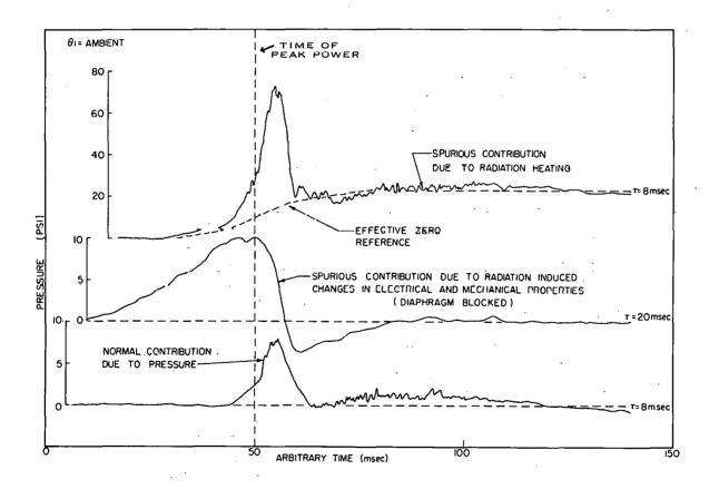
Fig. 6 Spurious output from a pressure transducer indicating the nature of transient and integrated radiation effects.
