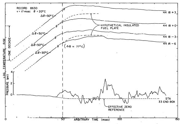
Fig. 18 A presentation of fuel-plate surface temperature-time histories at various longitudinal positions along a fuel plate and the pressure-time history. The symbol  $\theta$  on the temperature-time histories indicates the boiling temperature with the corresponding temperature rise shown in parentheses adjacent to one of the traces.
