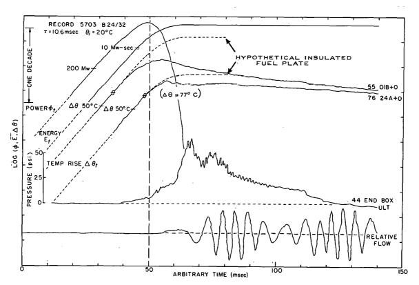
Fig. 108 A presentation of time histories for power, energy, fuel-plate surface temperature, pressure, and flow. The symbol  $\theta$  on the temperature-time histories indicates the boiling temperature with the corresponding temperature rise shown in parentheses adjacent to one of the traces.
