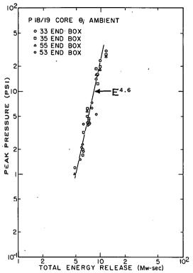
Fig. 37 Peak transient pressure in various lower end boxes as a function of total nuclear energy release for ambient initial temperature.
