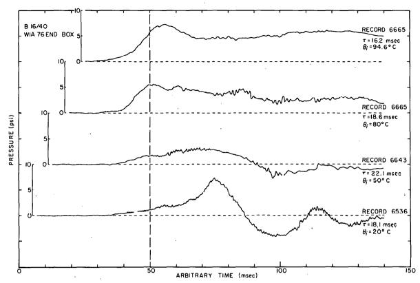
Fig. 127 Representative B 16/40 Core pressure-time histories for various initial temperatures.
