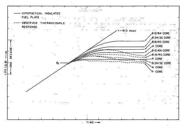
Fig. 146 Representative temperature-time histories and hypothetical insulated-plate behaviors for the Spert I cores.
