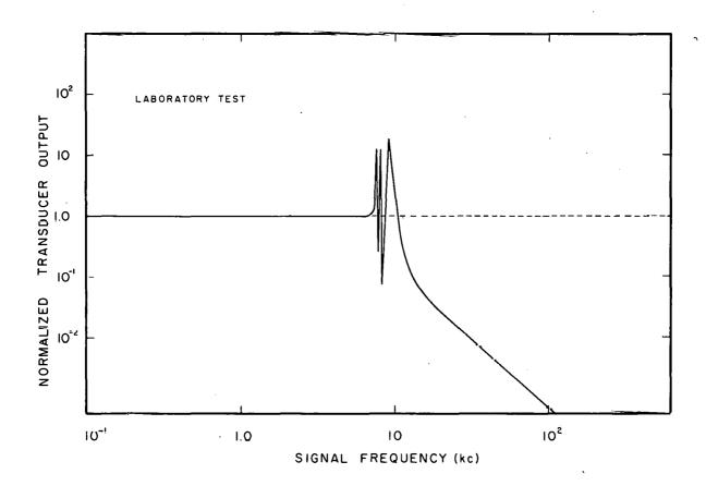
Fig. 8 Graphic representation of the response of a typical diaphragm-type transducer.
