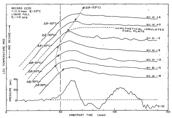
Fig. 51 A presentation of fuel-plate surface temperature-time histories at various longitudinal positions along a fuel plate and the pressure-time history for a specific initial pressure with the reactor vessel liquid full. The symbol  $\theta$  on the temperature-time histories indicates the boiling temperature with the corresponding temperature rise shown in parentheses adjacent to one of the traces.
