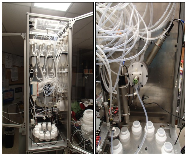
Fig. 2: The isotope harvesting end station designed to collect isotopes from the water dump currently used at MSU.
