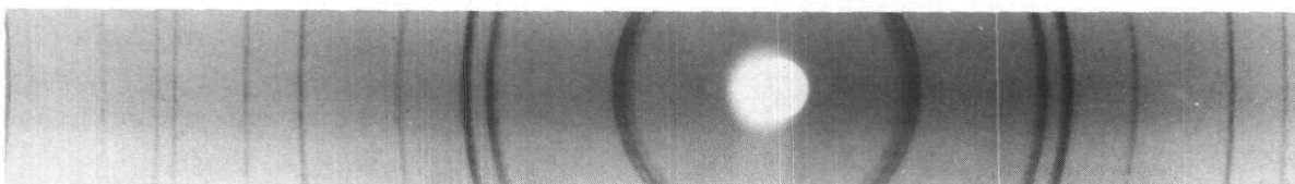
(a) Pu-44 a/o C. Quenched, 570^{\circ}\text{C} , 18 days (Microstructure showed coring)
