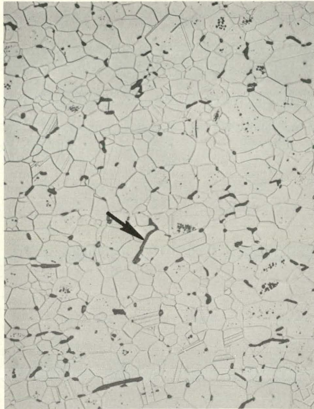
FIGURE 4. MICROSTRUCTURE OF 99% TD PELLET. ARROW INDICATES GRAPHITE PARTICLE. ETCHED IN 10% OXALIC ACID. 275X
