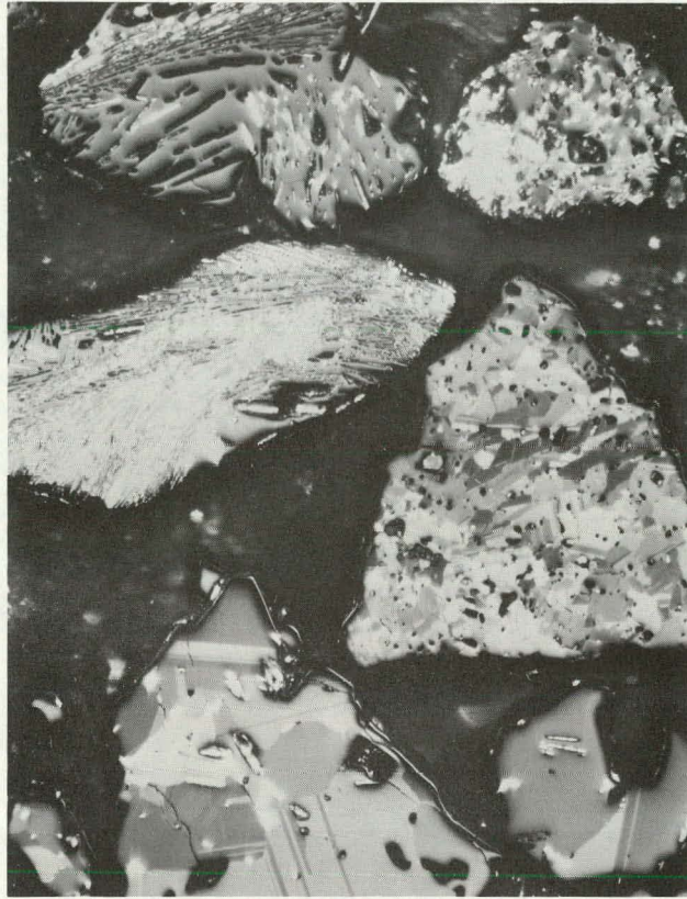
FIGURE 1. PREIRRADIATION B_4C PARTICLES. POLARIZED LIGHT. 32X
