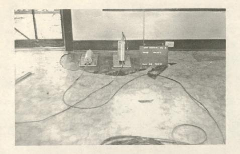
Photo #17: Station #4, Test House #4, seismometer location, north side of house.
