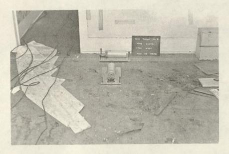
Photo #12: Station #3, Test House #3, seismometer location for Nov. 19, 1970, first floor center of house.
