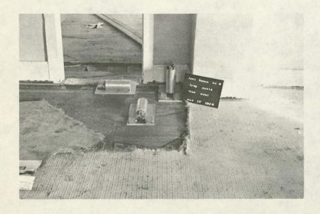
Photo #6: Station #2, Test House #2, seismometers on first floor, center of building.
