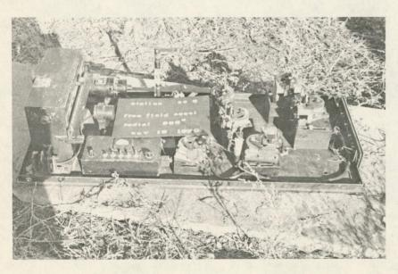
Photo #22: Station #6(free-field station), uncovered accelerograph, 3 components of acceleration (two levels).
