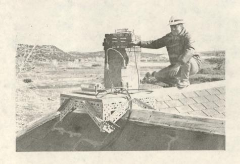
Photo #4: Station #1, Test House #1, looking northeast. Seismometers on roof and chimney.
