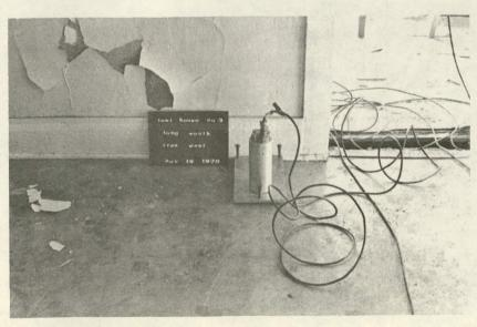
Photo #13: Station #3, Test House #3, seismometer location for Nov. 19, 1970, first floor south of the house.
