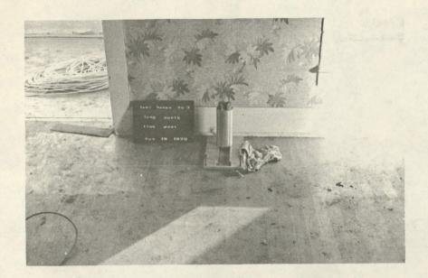
Photo #11: Station #3, Test House #3, seismometer location for Nov. 19, 1970, first floor, north side of house.
