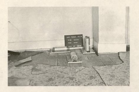
Photo #7: Station #2, Test House #2, Nov. 17, 1970. Seismometers located second floor, center of building.
