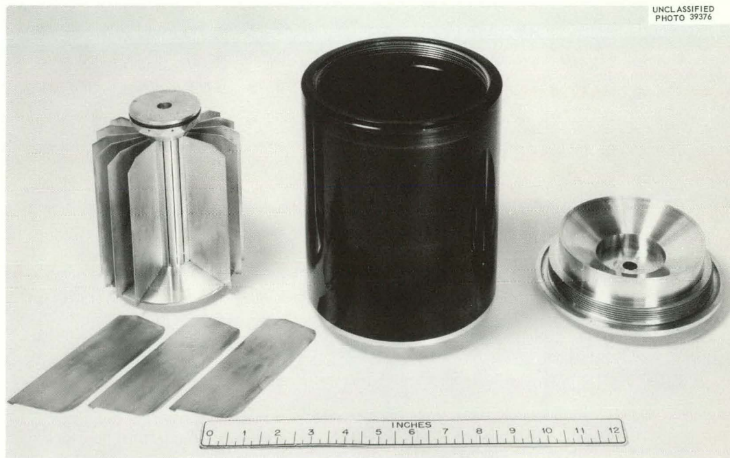
Fig. VI-C-1. Parts of Zonal Rotor B-III. Core assembly is shown on left, rotor body in center, and upper end cap at right. Gradient is static loaded through the center line leading from the upper end cap to the bottom of the core. When the gradient flows out the upper end cap annular constriction, the sample layer is forced back into the upper portion of rotor on top of gradient. Gradient is recovered by pumping dense fluid to bottom of chamber at rest, forcing gradient out top.
