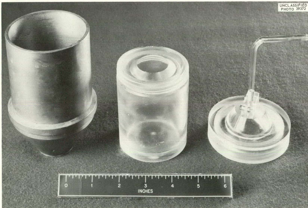
Fig. X-B-2. Rotor F-I-f, with Transfer Cap Shown. When assembled, it is rotor F-II-f.
