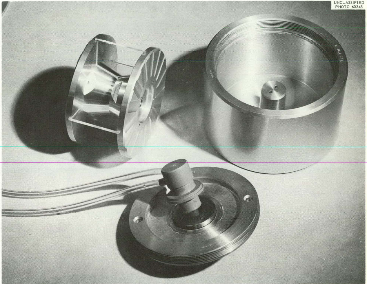
Fig. II-B-5. Zonal Rotor A-IV. Rotor used to demonstrate gradient introduction and recovery from rotor at speeds up to 18,000 rpm. Used in Spinco Model K centrifuge.
