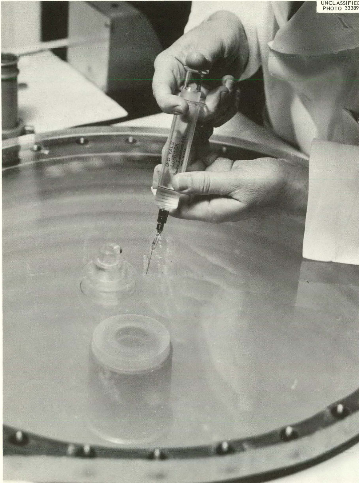
Fig. X-B-4. Technique for Ultrarapid Freezing of Cells by Injection into Liquid Nitrogen into Rotor F-I-f.
