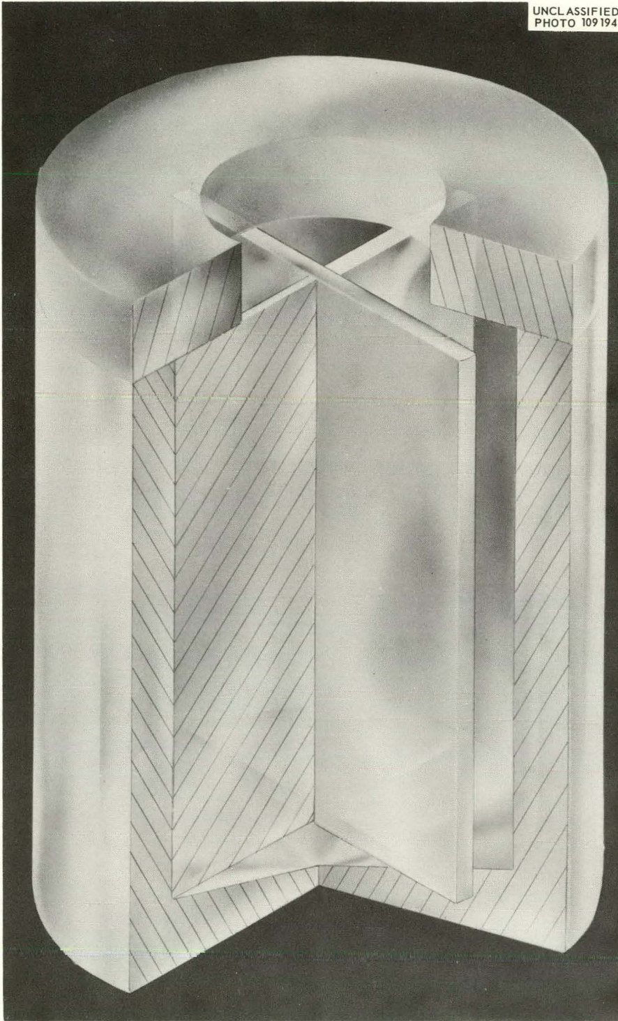
Fig. V-C-1. Drawing of Rotor A-VII. The hollow interior is divided into four sector-shaped compartments by vertical septa. The shallow conical bottom extends below the septa. Filling and emptying is through a narrow tube inserted through the top opening to the bottom of the rotor. At 3000 rpm the gradient extends from the edge of the rotor only as far in as the edge of the center upper hole. The gradient does not, therefore, completely fill the rotor at rest. A rubber stopper is inserted to minimize effects of air friction during operation.
