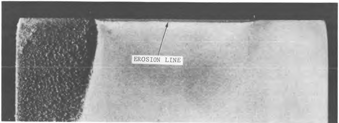
FIGURE 6-10. PHOTOGRAPH OF TEST WEDGE 4, 120° SIDE
