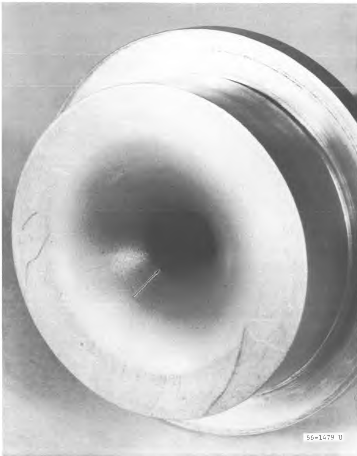
FIGURE 6-14. PHOTOGRAPH OF TEST NOZZLE 2 SHOWING DEPOSITION PATTERN ON SUBSONIC PORTION OF NOZZLE
