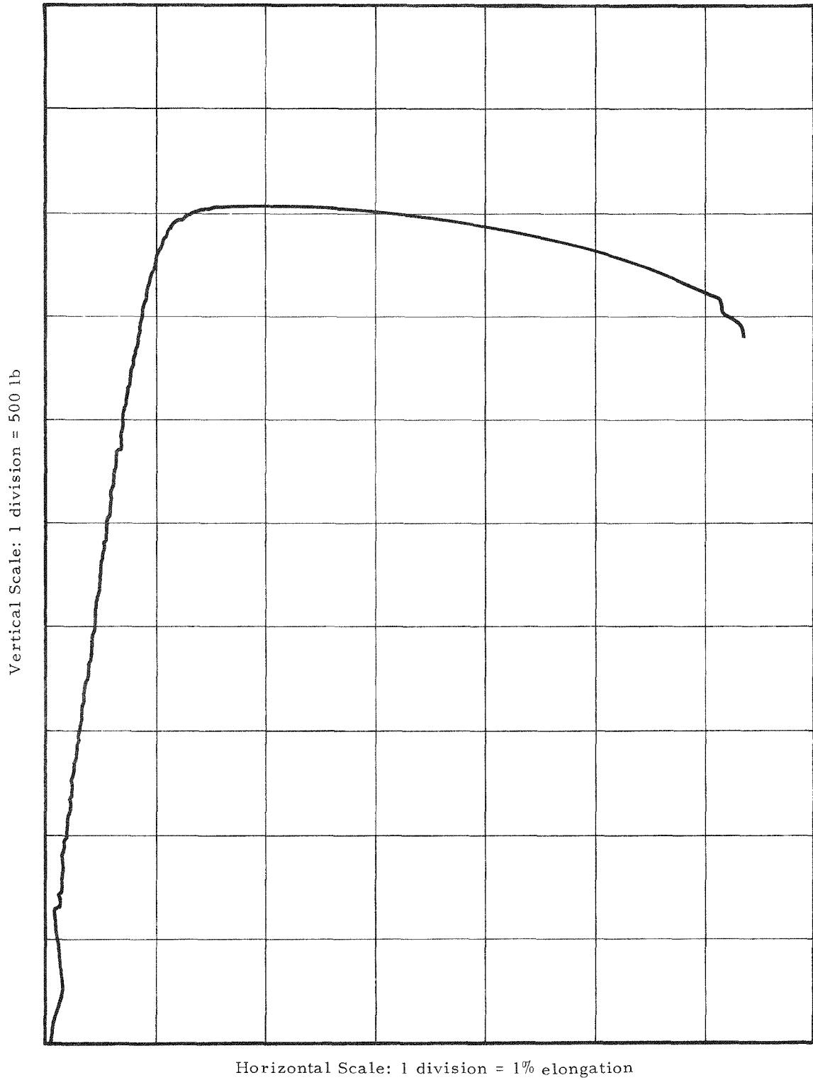
Figure 7-3. Load Deflection Curve for a Specimen Tested at 70 F
