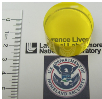
Figure 2. Photograph of a 3.2 cm diameter by 2 cm tall \text{YGAG}(\text{Ce}) ceramic. This composition possesses the excellent phase stability required in order to avoid secondary phases that lead to deleterious scatter. This sample exhibits optical scatter \alpha < 0.1\text{ cm}^{-1} .
