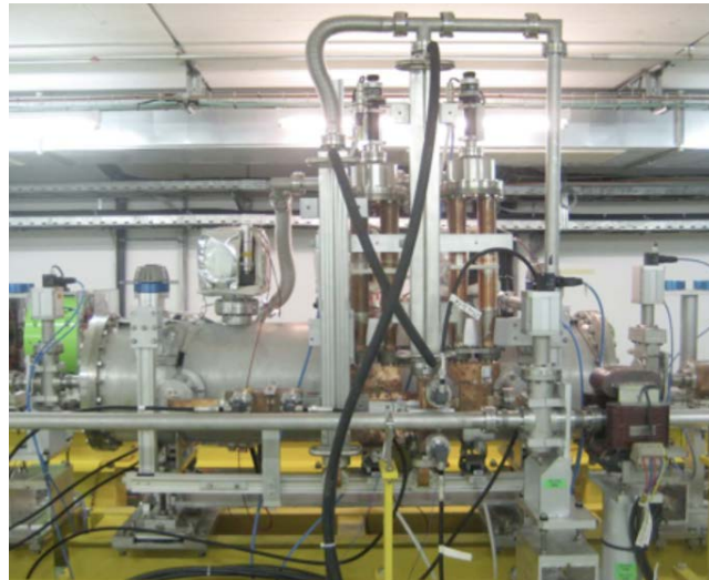
Fig. 7.15: The TBTS PETS tank with the power recirculator installed, including the variable power splitter and phase shifter
