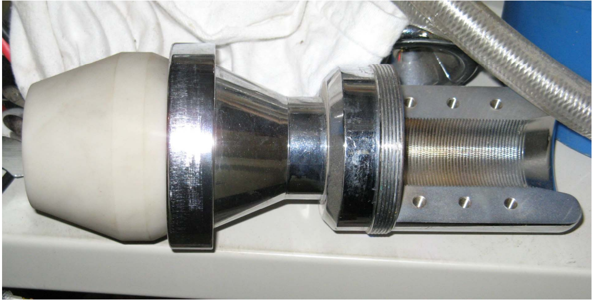
Fig. 5.262: New feedthrough connector developed at KEK/ATF
