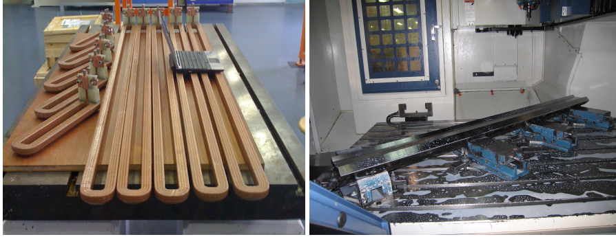
Fig. 5.6: Main Beam Quadrupole prototype procurement: coils and iron quadrant (during machining)
