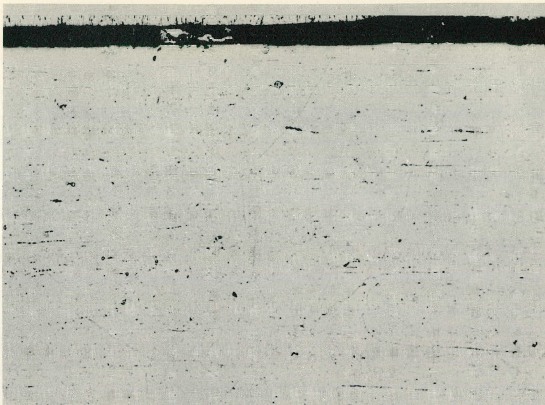
Fig. 11 Y-19068 250 X Compression side of tube number 1 from the NaK inlet header. Note the absence of voids as compared with Figure 10. Etched with electrolytic oxalic acid.
