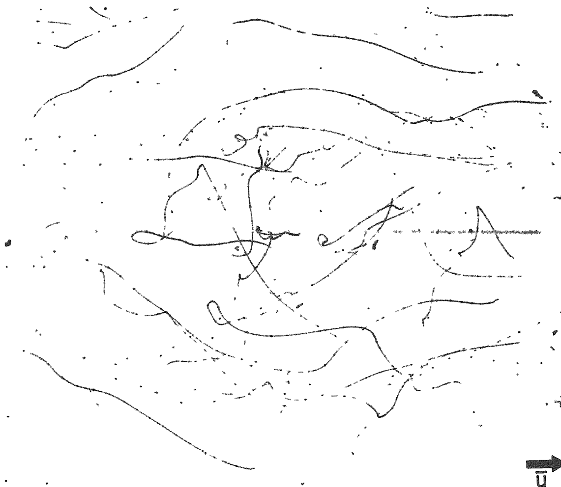
Fig. 6.--Positive reversal of 17-sec long turbulent trajectories photographed from above in experiment S/25/y; horizontal line is the drive cable; droplets are moving in direction of the arrow.
