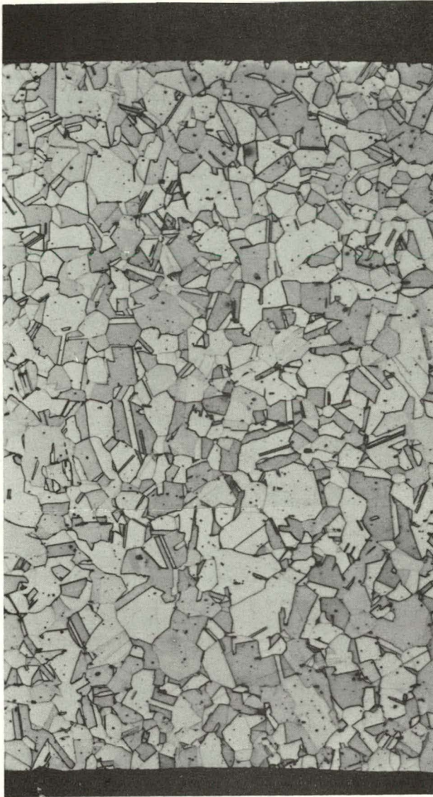
AS-RECEIVED TUBING, MODIFIED GLYCEREGIA ETCH, 250X
