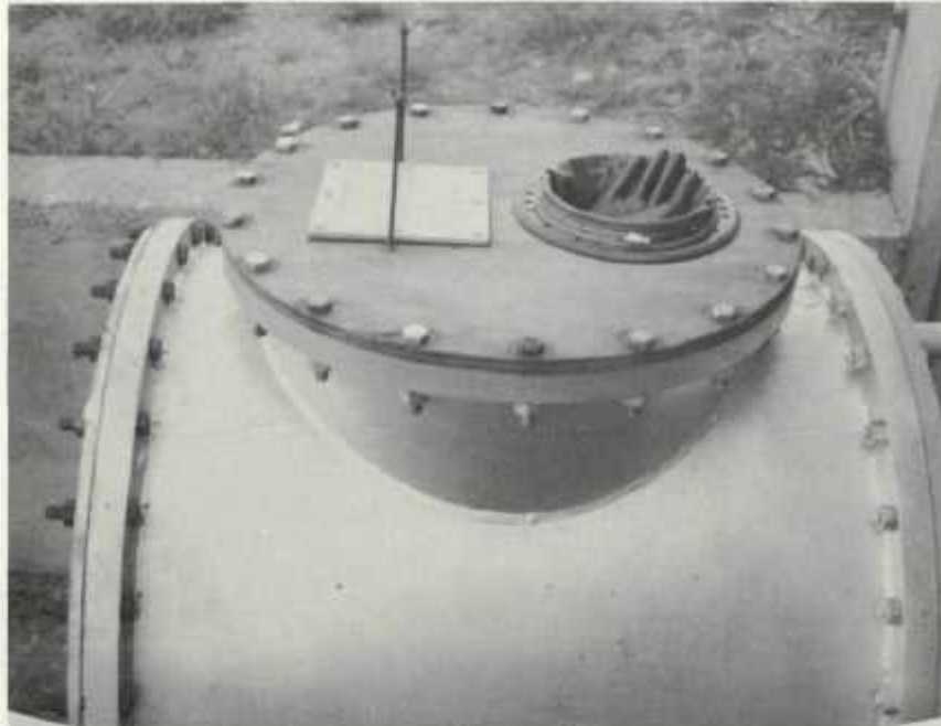
FIGURE 5-2 - MOUNTING OF GLOVES ON THE 3ft x 3ft CYLINDRICAL TEST CHAMBER (Arrangement A)
