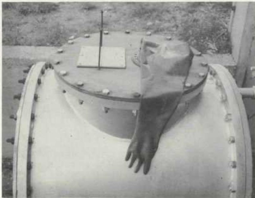
FIGURE 5-3 - MOUNTING OF GLOVES ON THE 3ft x 3ft CYLINDRICAL TEST CHAMBER (Arrangement B)
