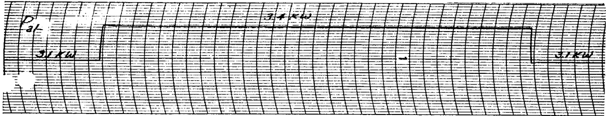
FIG 45 CONTROL ANALYSIS \frac{P_{out}}{N(s)} = \frac{10}{(1+0.2s)^2} WATTS / RPM
