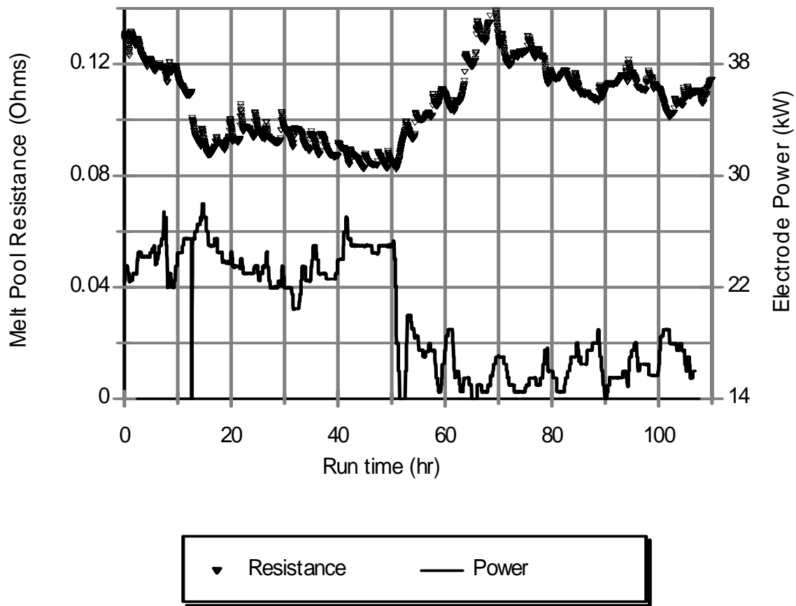
Figure 4.6.c. Melt pool resistance and total electrode power during DM100 Tests 5 and 6.
