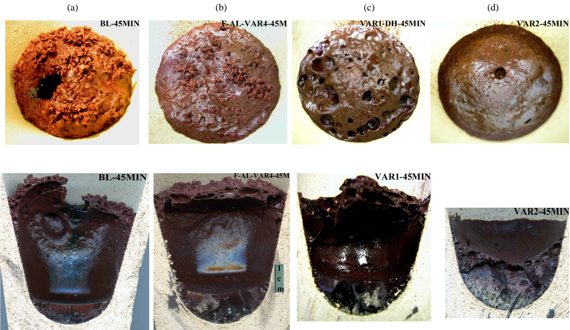
Figure 3.6. Impacts of boron and aluminum sources on melt rate in VGF experiments (45 minutes). (a) \text{Al}_2\text{O}_3 and borax, (b) \text{Al}(\text{OH})_3 and borax, (c) \text{Al}_2\text{O}_3 and boric acid, and (d) \text{Al}(\text{OH})_3 and boric acid
