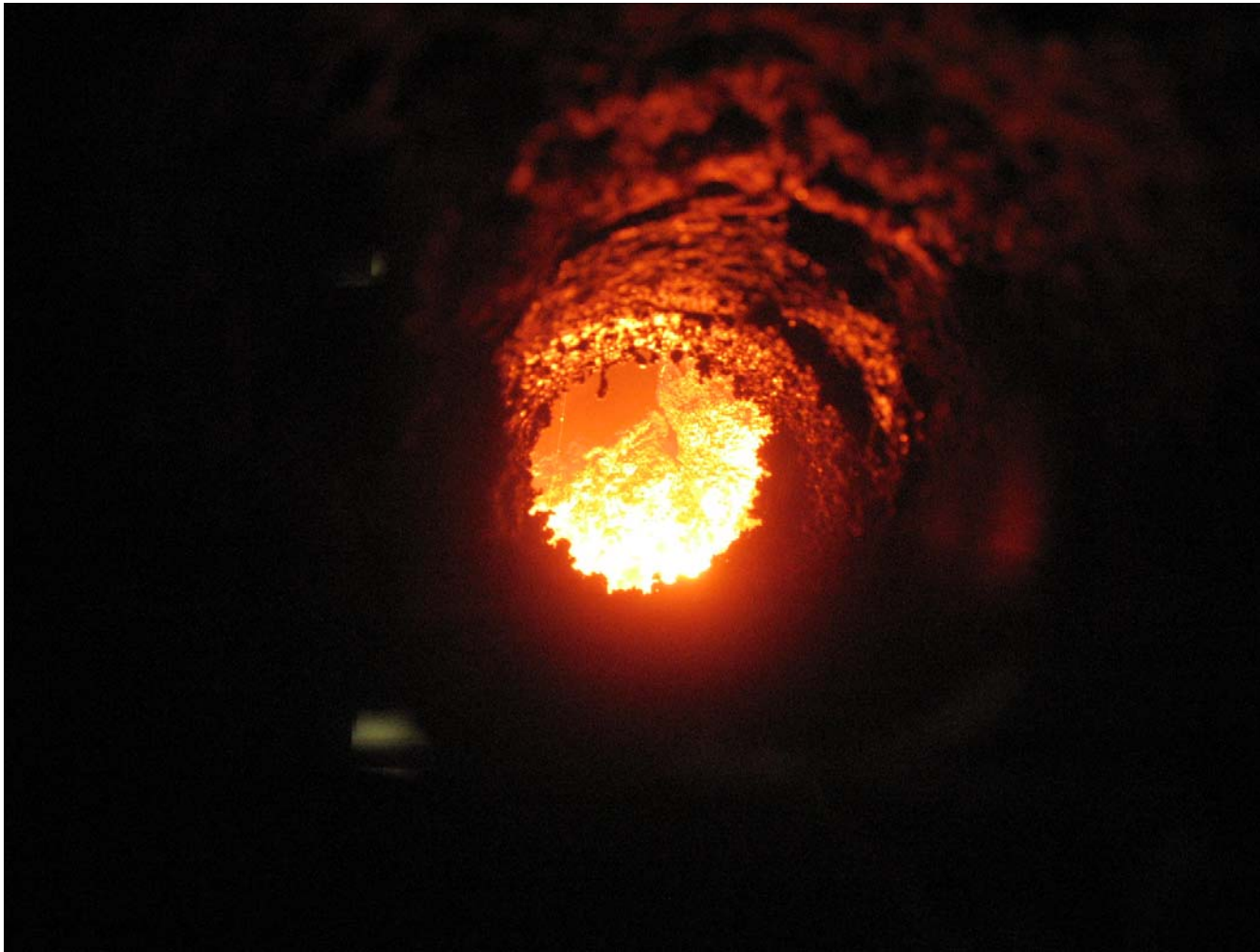
Figure 5.1. Picture of cold cap through north view port showing the thickness of the cold cap.
