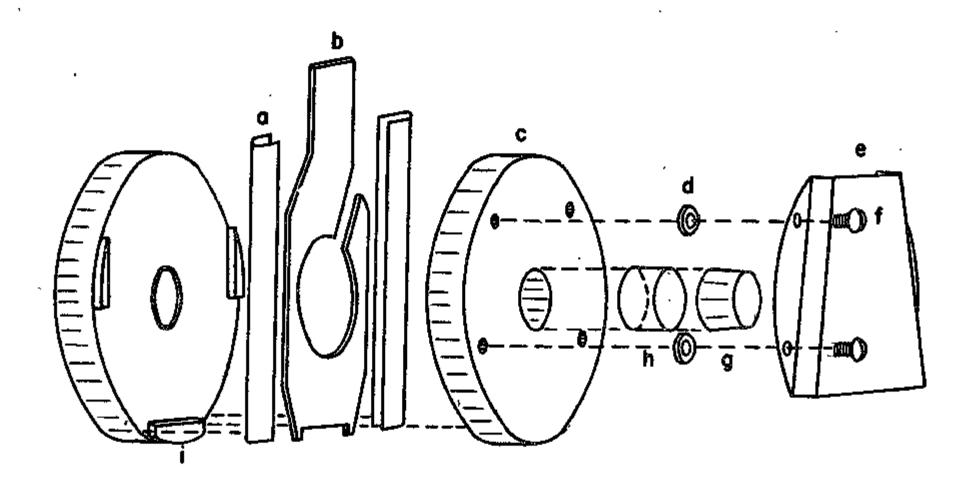
Figure 4: Capacitance Cell Assembly Cross Section
