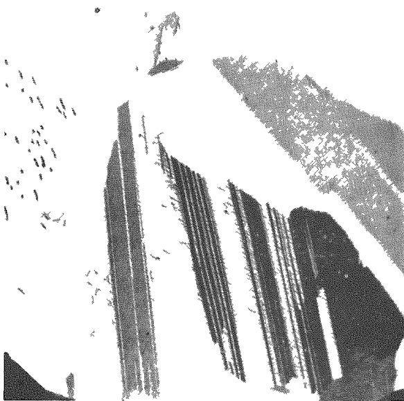
Uranium-8.5 w/o Carbon As Cast
