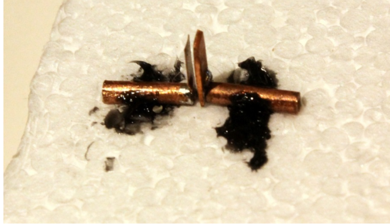
Figure 108. Experimental prototype of mechanically modulated dipole antenna
