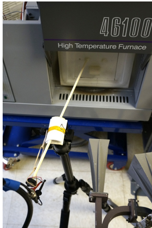
Figure 172. Alumina rod used to directly excite Pt/alumina sensor. A piezoelectric transducer attached to one end of rod was used to launch acoustic waves into rod. The other end of the rod was held in contact with the alumina bolts used to mount the sensor to the Zircar insulating plate.
