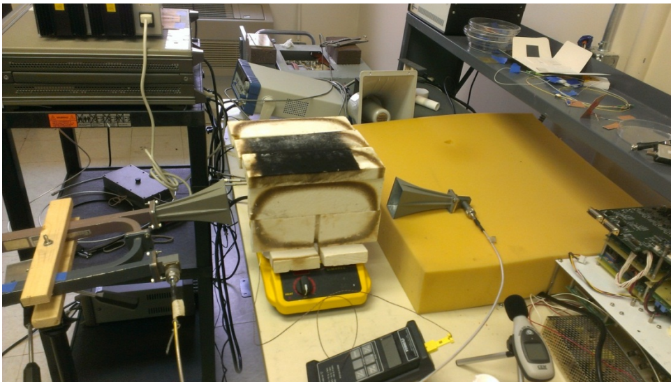
Figure 176. Experimental set-up used to measure temperature dependent microwave attenuation of Zircar alumina panel with temperature.
