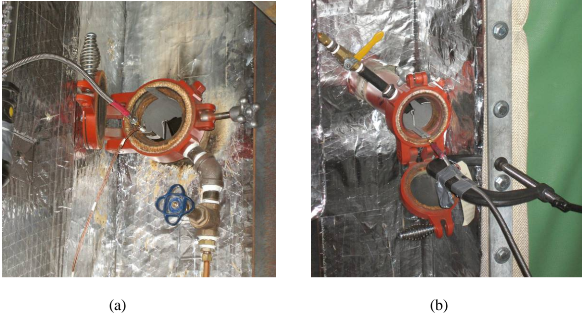
Figure 139. Photographs of (a) Antenna A and (b) Antenna B installed in viewports in the SBS.
