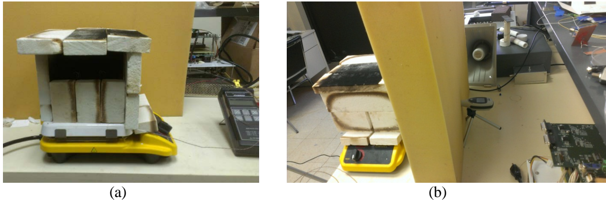
Figure 175. Test set-up to determine temperature sensitivity of acoustic attenuation of Zircar alumina
