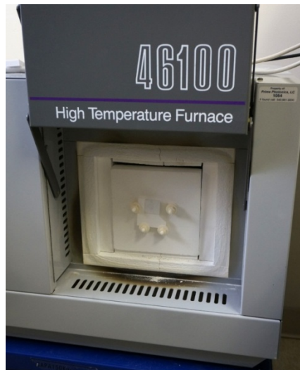
Figure 165. Zircar refractory panel in face of Thermolyne high temperature furnace. The DBC sensor can be seen held in position with alumina hardware. For high temperature tests, the Zircar panel was rotated so that the sensor was in the interior of the furnace cavity.
