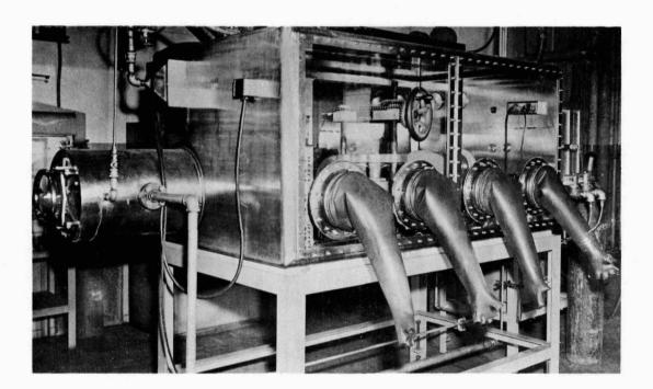
Figure 2 - Glove box for work on refractory uranium compounds.
