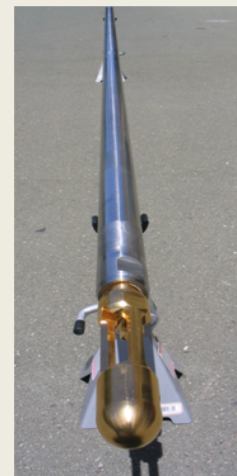
Thermochem Downhole Sampler (DHS); Useful to ~350°C for several hours
