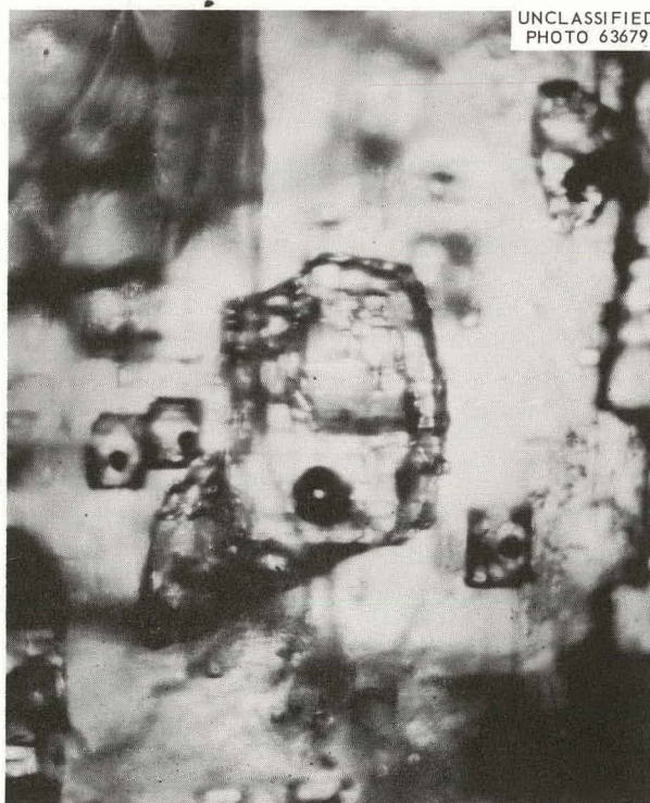
Fig. 4.7. Liquid Inclusion in Rock Salt. Reduced 17%.
