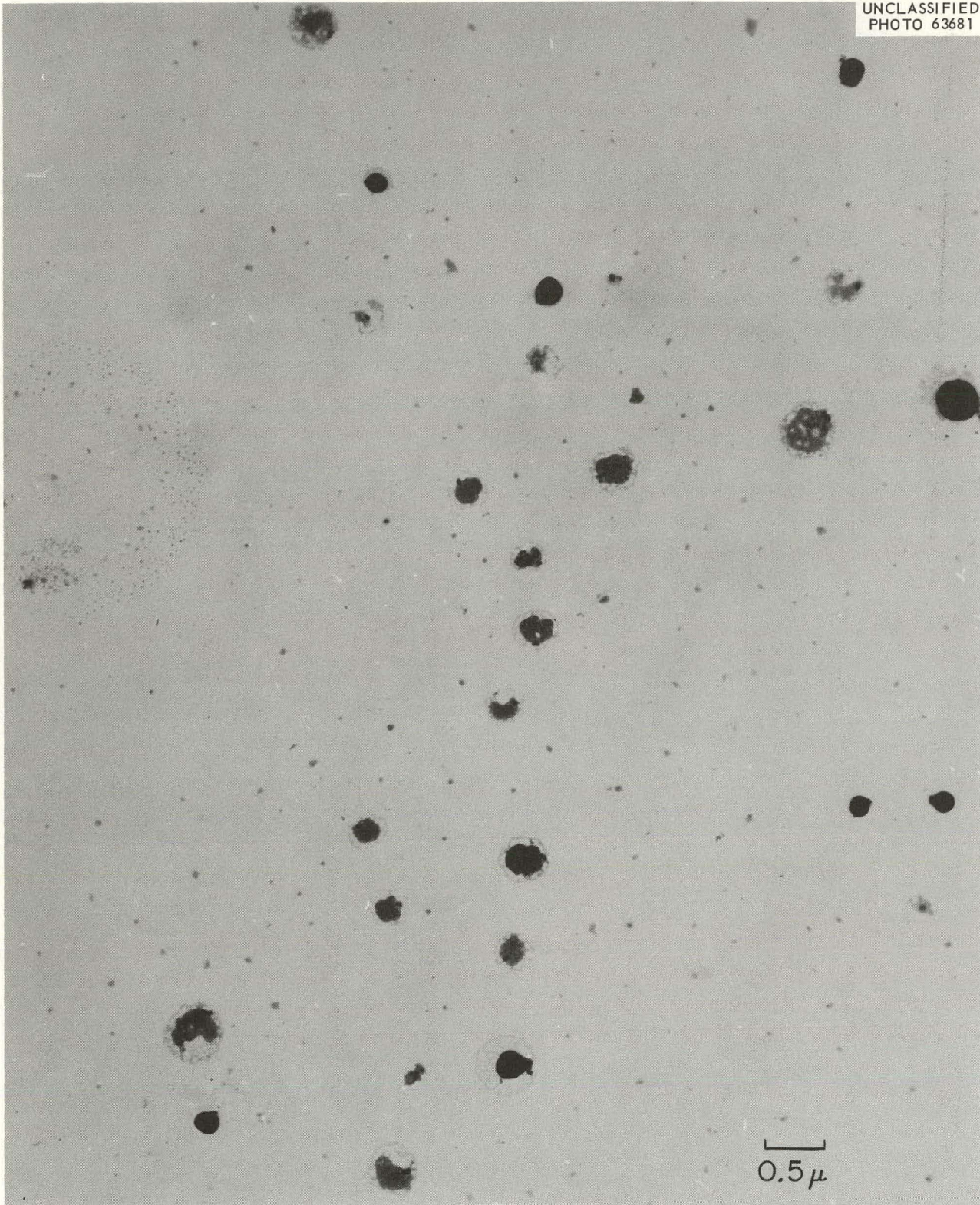
Fig. 10.3. Particles Collected by the Electrostatic Precipitator in Line During the Fission Product Release Experiment.
