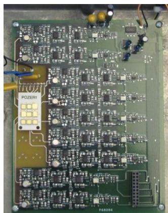
Figure 12. Nine-channel COTS readout integrated with nine-element Pillar Detector array.
