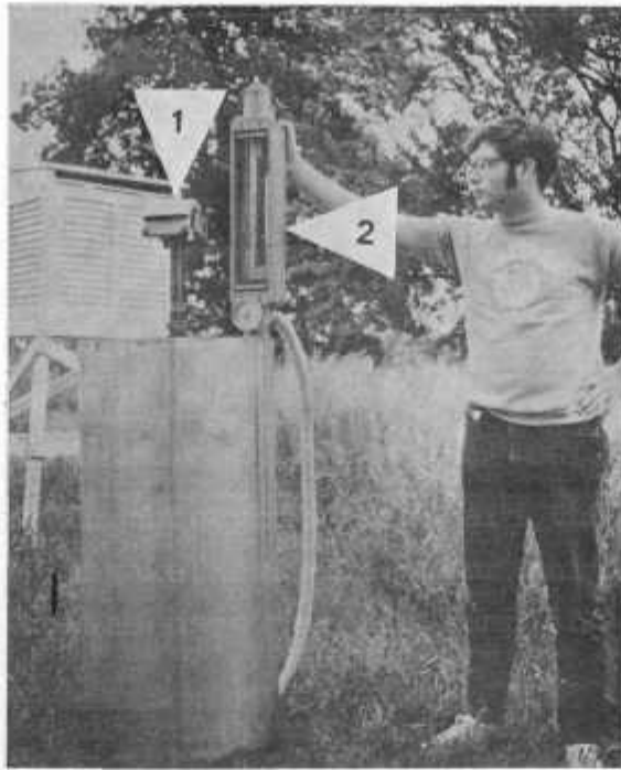
Figure 2. Hi-volume air sampler, supplied by Argonne National Laboratory for use at the base station. Indicated in the photograph are the (1) intake and (2) flow rate meter.
