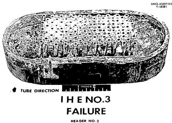
Fig. 133. Bottom Side of IHE No. 3, NaK Outlet Head, Showing Bending of Tubes.
