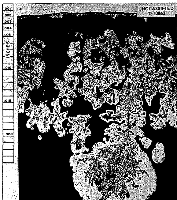
Fig. 55. Deposits Found in Inconel Pump Loop 7426-12 Operated with Sodium at 1500°F. 150X. Reduced 22%.
