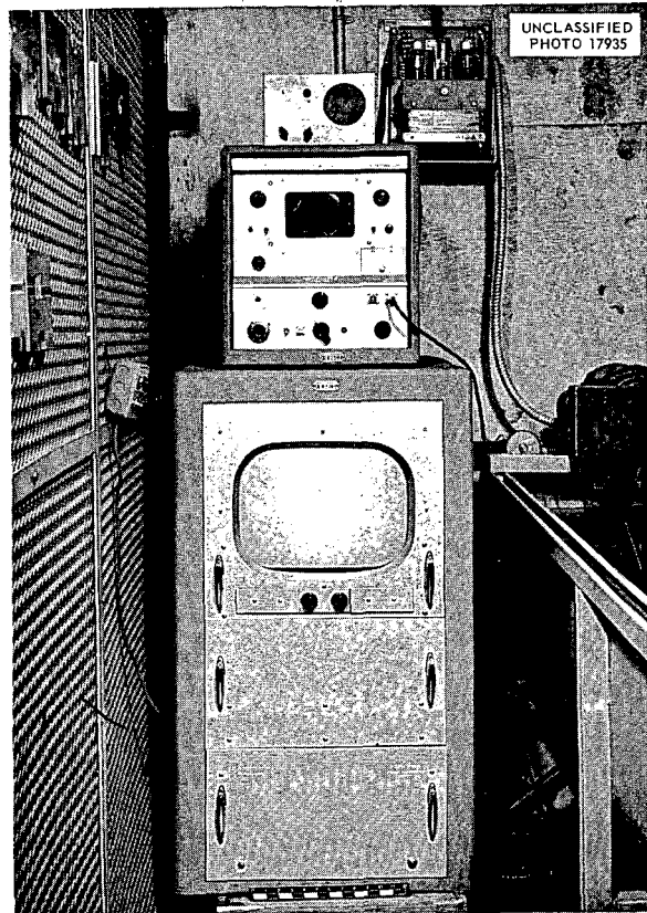
Fig. 94. Instrumentation for the Immersed Ultrasonic Inspection of Pipe.
