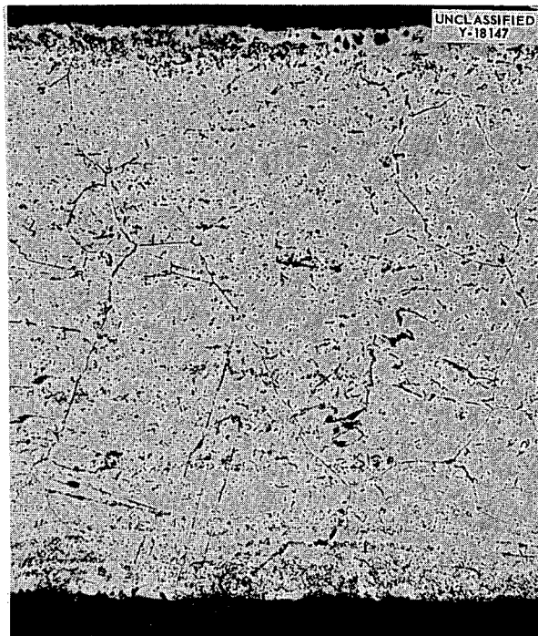
Fig. 198. Inconel Tube Wall in Area C. Note small amount of subsurface voids on fuel side (top of photomicrograph) and absence of intergranular attack on NaK side (bottom). Note uniform distribution of precipitate. 250X. Reduced 26.5%. (Confidential with caption)
