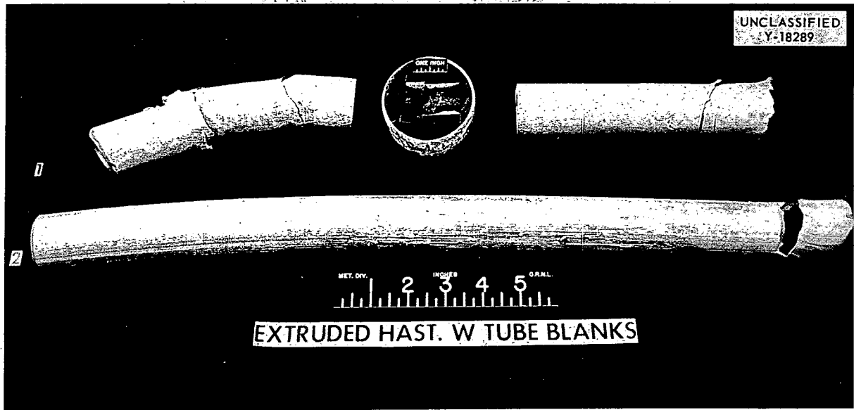
Fig. 151. Seamless Tube Blanks Extruded from Forged Hastelloy W Billets Canned in Inconel. Tube 1 was extruded at a fast rate at 2100°F. Tube 2 was extruded slowly at 2200°F.
