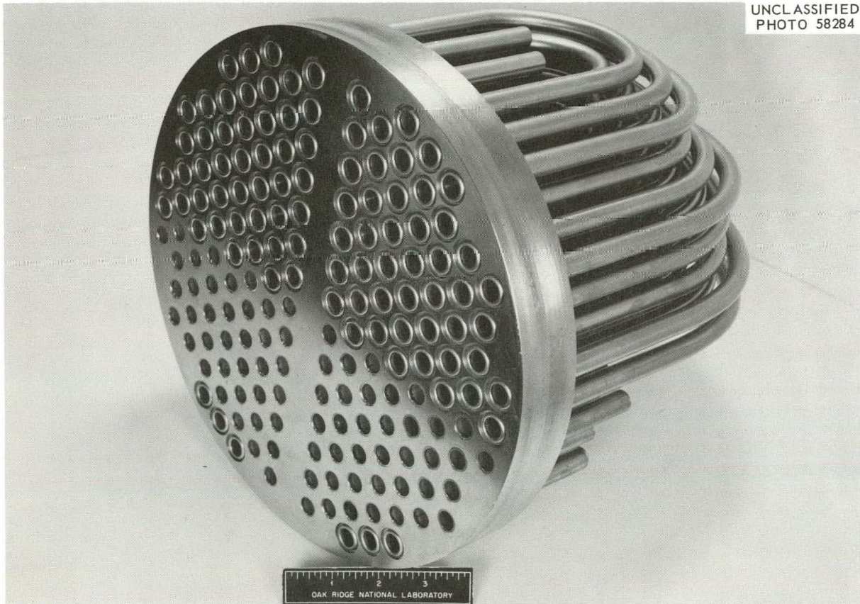
Fig. 7. Proof-Test Assembly Containing Short U-Tubes.
