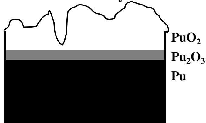
(b) Scratched oxide layer (note the scratch through Pu 2 O 3 )
