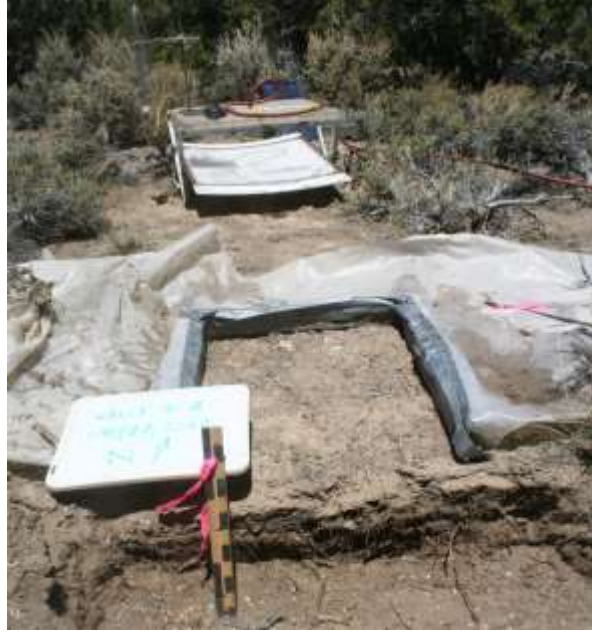
Figure 8. Photograph of portable rainfall simulator (background) before installation over area to be sampled (foreground). The Plexiglas plate beneath the simulator is for rainfall collection for calibration. Trench for collection trough at the downstream side of plot is also shown.
