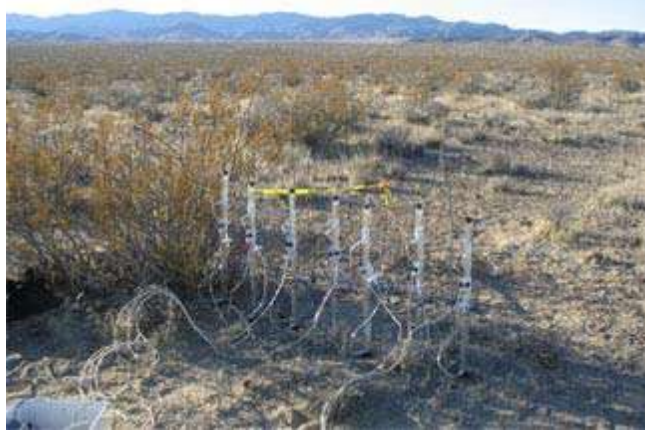
Figure 7. Set of eight modified MDTIs linked to a datalogger.
