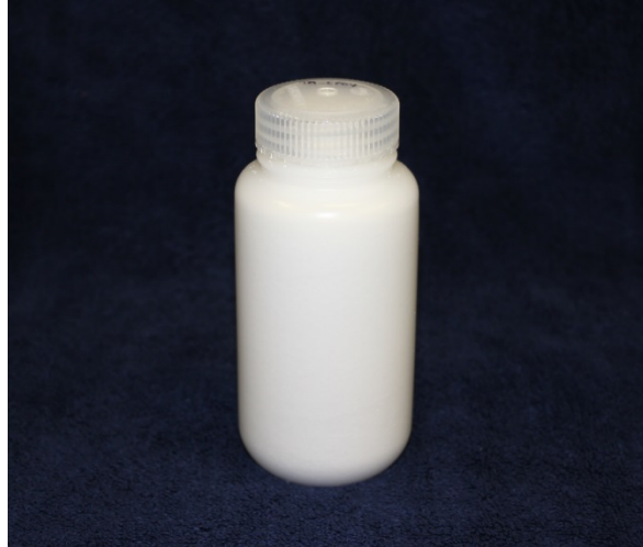
Figure 6. Example specimen consisting of a 250-ml Nalgene specimen bottle packed with tartaric acid.
