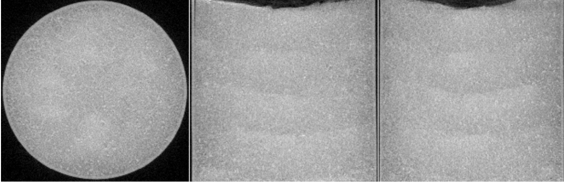
Figure 8. Reconstructed CT images of TA_SH01 scanned on the single-slit MicroCT. A horizontal midsection image is at left and two orthogonal vertical images are center and right. The specimen slit for dual-slit MicroCT covers the bottom ~2% of the vertical images.
