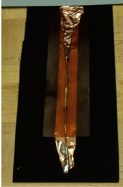
Figure 6.1. View of a complete capillary tube assembly, showing the powder-filled volume at the very center, the copper wire inserted into both ends of the tube, and the copper foil source strip (top) and return (backplane), with Kapton sheet used as insulation.
