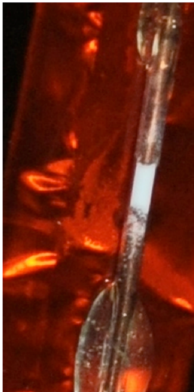
Figure 6.2. Close-up view of the powder-filled volume. The clear blobs at top and bottom are the epoxy used to hold the copper wire in place.
