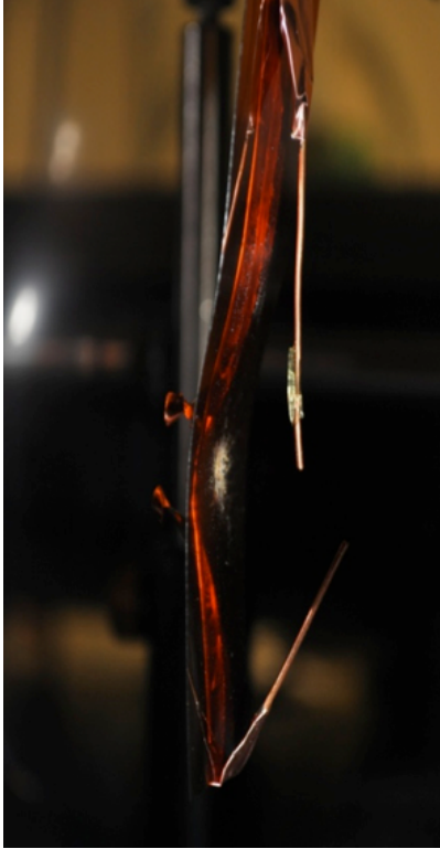
Figure 6.7. Post-shot photograph of a PETN test, showing destruction of the capillary and deformed of the copper backplane. The white blur in the middle is scoured Kapton, not powder residue; Raman spectroscopy confirmed the absence of PETN.
