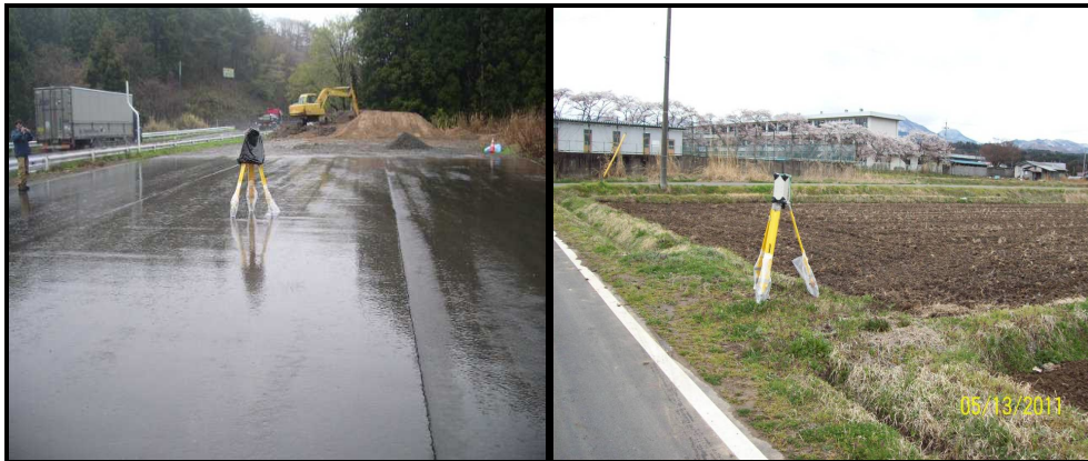
Figure 3. Examples of less-than-ideal in situ site selection – inhomogeneous surfaces and those prone to runoff complicate radionuclide assay, whether for detection limits, nuclide deposition concentrations, or activity ratios.
