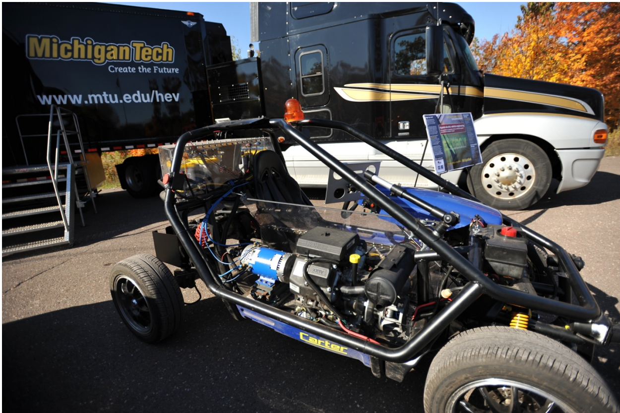
Figure 12: The Mobile Lab's Configurable Hybrid Electric Vehicle (CHEV) allows students to change virtually all aspects of the vehicle, and assess those changes on vehicle performance.
