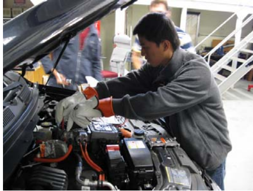
Figure 1: Student testing for the presence of high voltage in the Introduction to Propulsion Systems for Hybrid Electric Vehicles" lab course.
