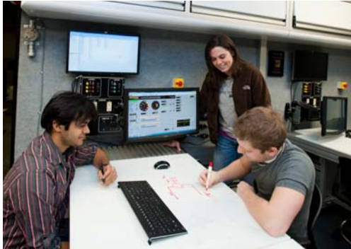
Figure 8: The universal lab benches are on wheels and employ T-Slots and removable dry erase hard surfaces
