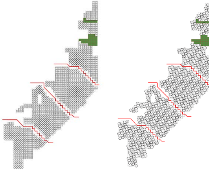
Figure ES5. New Jersey area of analysis and layout maps of the four leasing area delineation for the 8 D x 8 D spacing with a zero-degree grid orientation (left) and 10 D x 12 D baseline spacing with a 75-degree grid orientation (right) (Source: NREL)
