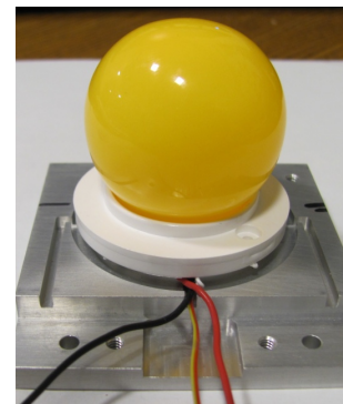
Fig. 2. Year 1 prototype ~1000 lm LED package with integrated remote converter. The prototype was mounted on a metal test fixture.
