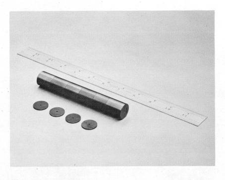
Figure 5. Thorium Metal Sample Including Buffer Pieces and Cooling Jacket
