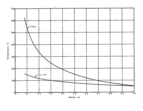
Figure 1. Temperature Distributions in Thorium Metal and Oxide Rods ( $P_{\ell}$  = 100 watts/cm)
