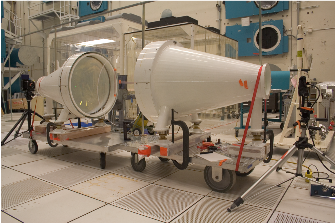
Figure 2.2: Prototype Schlieren imaging system for phase object screening
