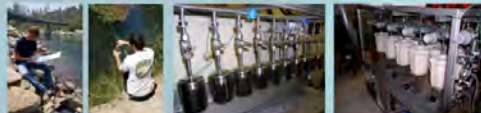
In the field, sampling and recording water quality parameters. Samples hanging on manifold for degassing under vacuum. Samples kept frozen with dry ice after cryogenic separation of 3 He gas from water.
