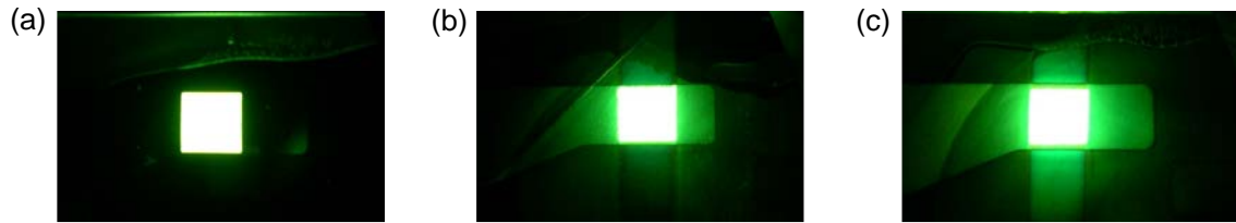
Figure 14. Emitting images of (a) the reference, (b) 70°C-cured, and (c) 40°C-cured grating devices, respectively, driven at the same current density.
