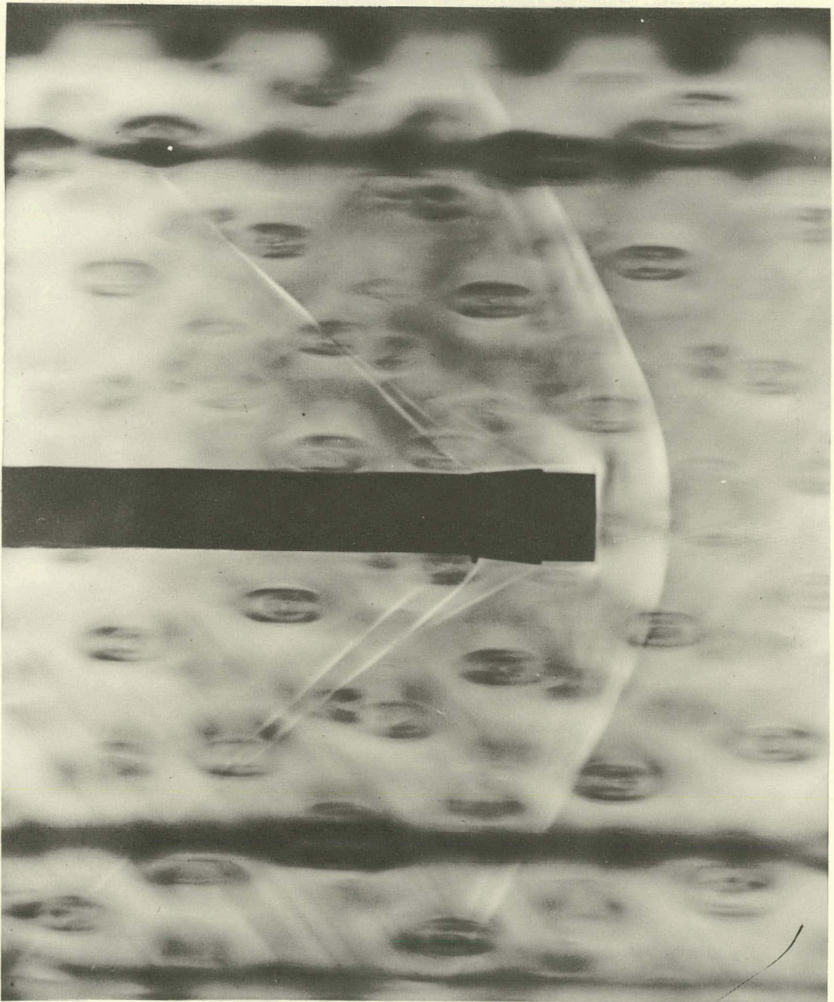
Figure 3. Bluff body (0.60 inch diameter) at M = 1.30 --Sandia Corporation 12 x 12 inch transonic wind tunnel
