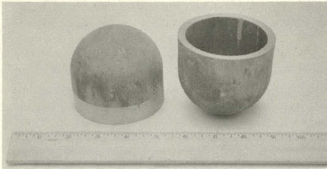
FIGURE 22. Typical experimental as-formed beryllium parts formed on Type-1 tooling (Figure 19). The cylindrical skirts are removed by trepanning and are machined to rings. The part on the left is partially machined. Light lines on the inside surface of the part at right resulted from severe ironing.
