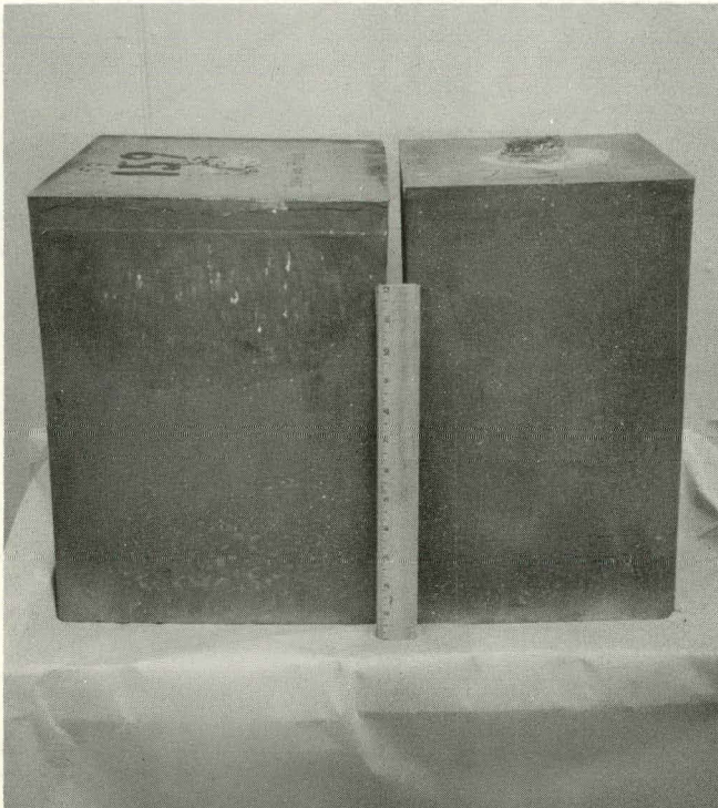
FIGURE 6. Two large rectangular as-cast ingots—the casting on the left measures 11 by 11 by 15.5 inches; the one on the right measures 9 by 9 by 15.5 inches.
