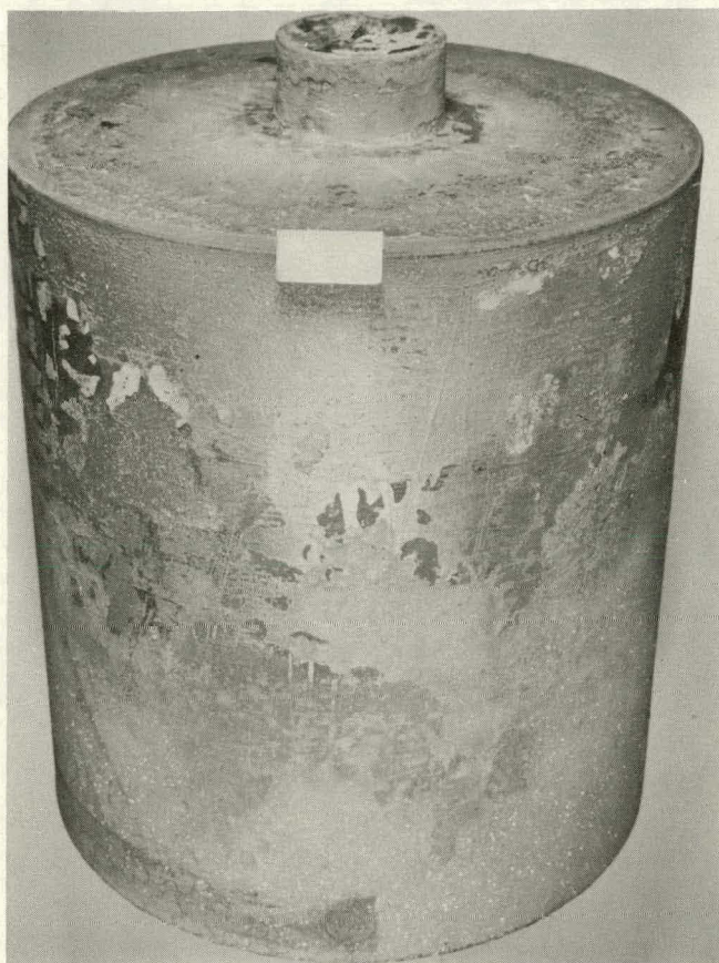
FIGURE 8. As-cast beryllium ingot, 7-inch diameter, 12.5 inches high. Large surface grains are the result of variations in mold coating, which acts as a thermal barrier.
