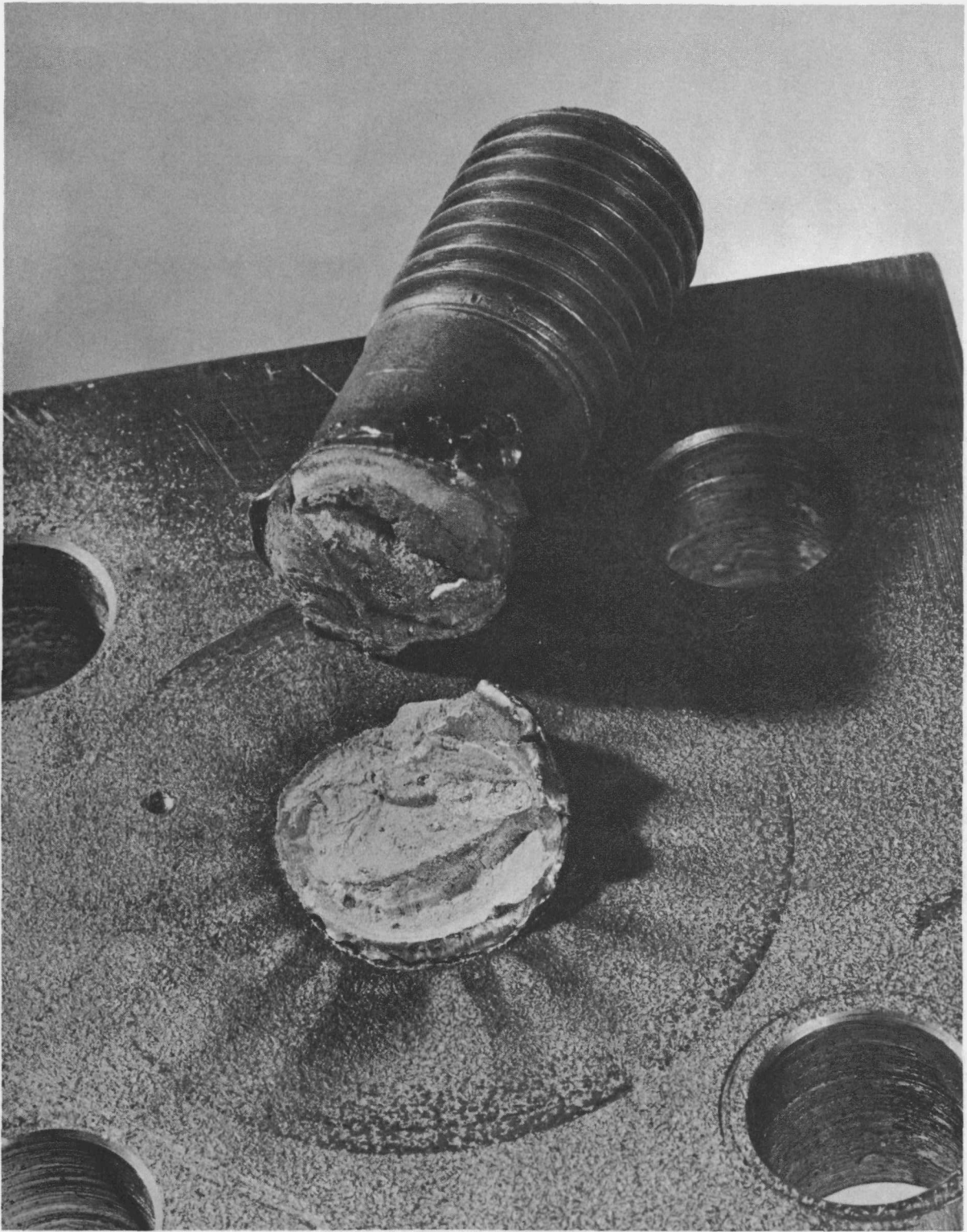
Fig. 1.12--Typical failure of 3/4-in.-diameter stud
