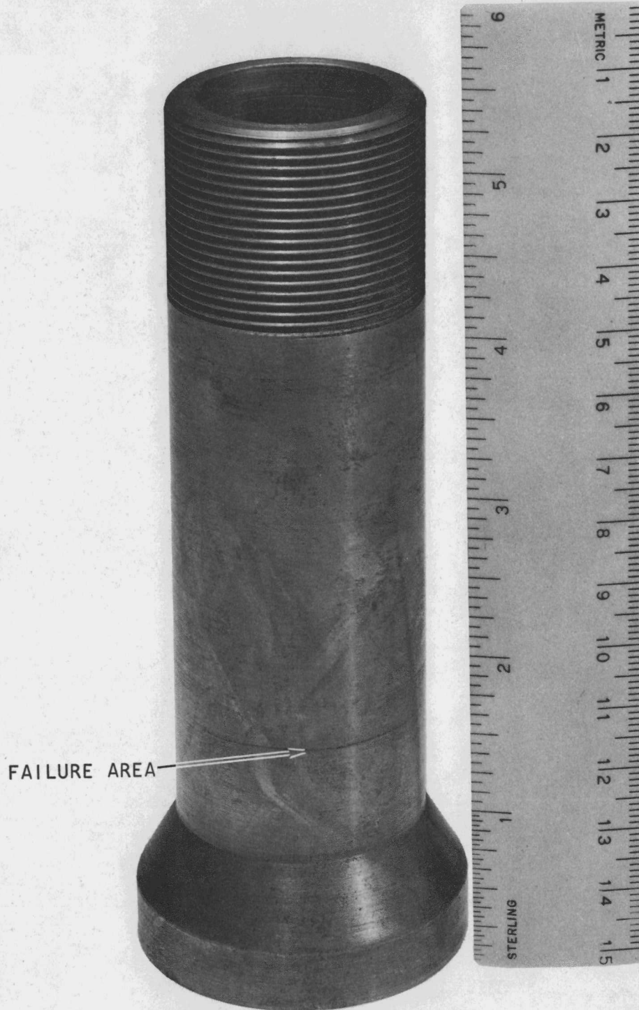
Fig. 1.13--Typical failure at wall thickness transition point (see Fig. 1.5)
