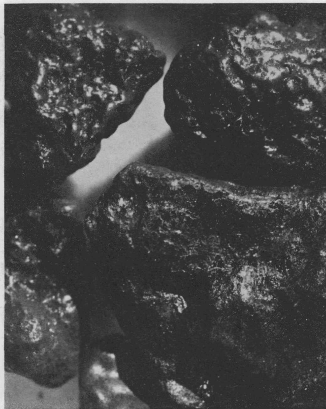
Fig. 3.8--Uncoated B 4 C granules 1/4- to 1/8-in. diameter (3471-106): prior to vibration test (left) and after vibration test of 1000 hr, 60 cps, 12-g maximum acceleration (right) (10X)
