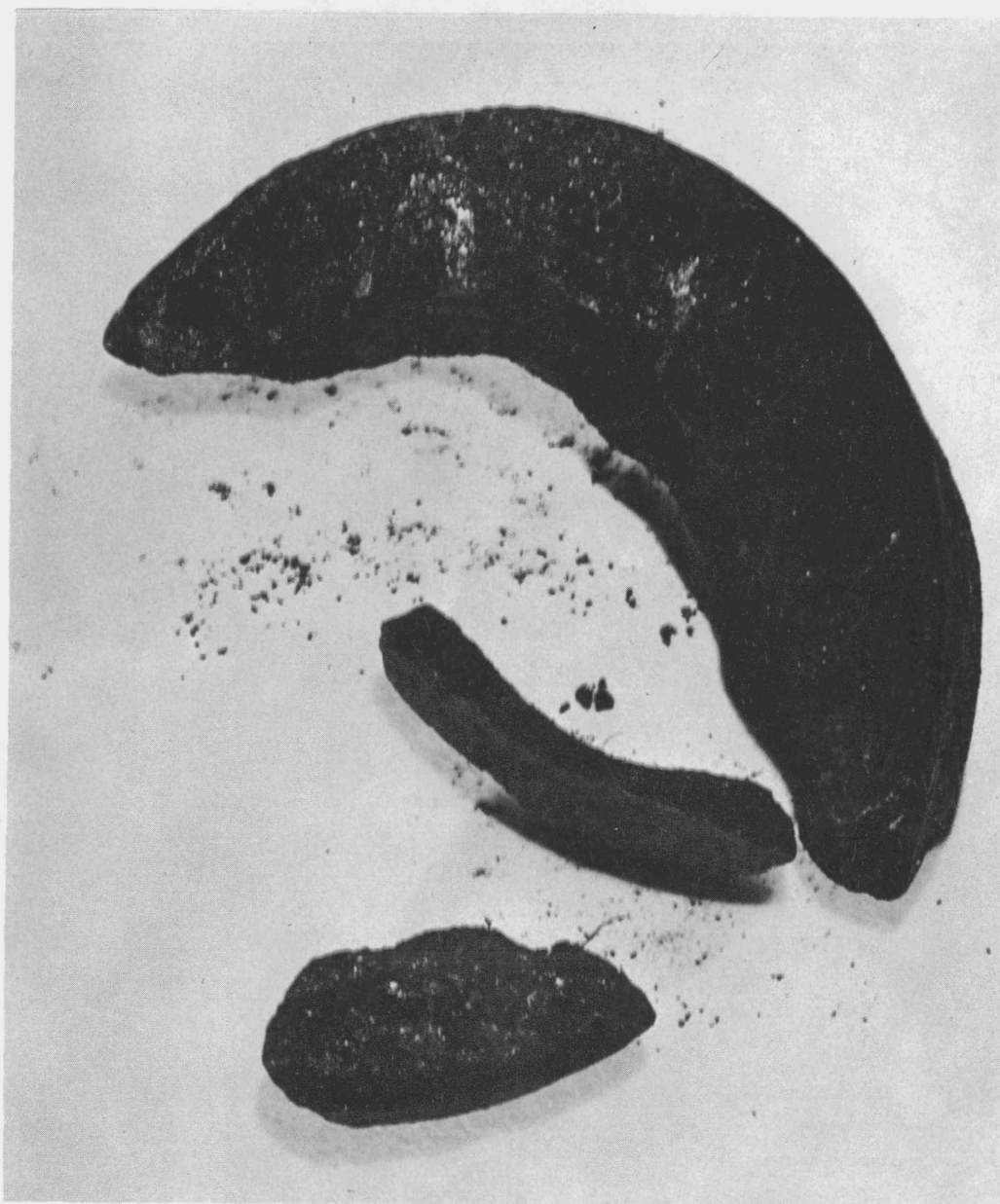
Fig. 3.7--Compacted wear dust formed at the bottom of the bed of PyC-coated B_4C after a 1000-hr vibration test ( \sim 6X )
