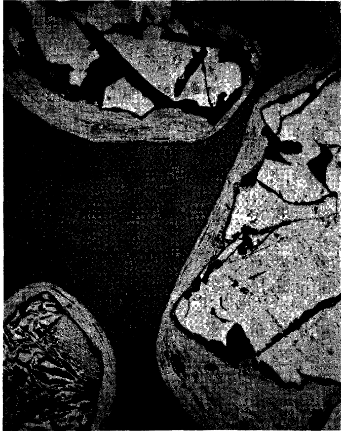
Fig. 3.10--PyC-coated B 4 C (3507-57-19) before (left) and after (right) vibration tests of 1000 hr, 60 cps, 12-g maximum acceleration (50X)
