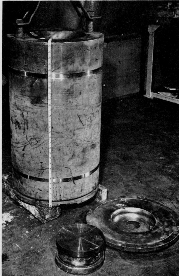
FIGURE 2 Copper Crucible for 7-Inch Diameter Ingot with Copper Base Plate and Uranium Starting Pad
