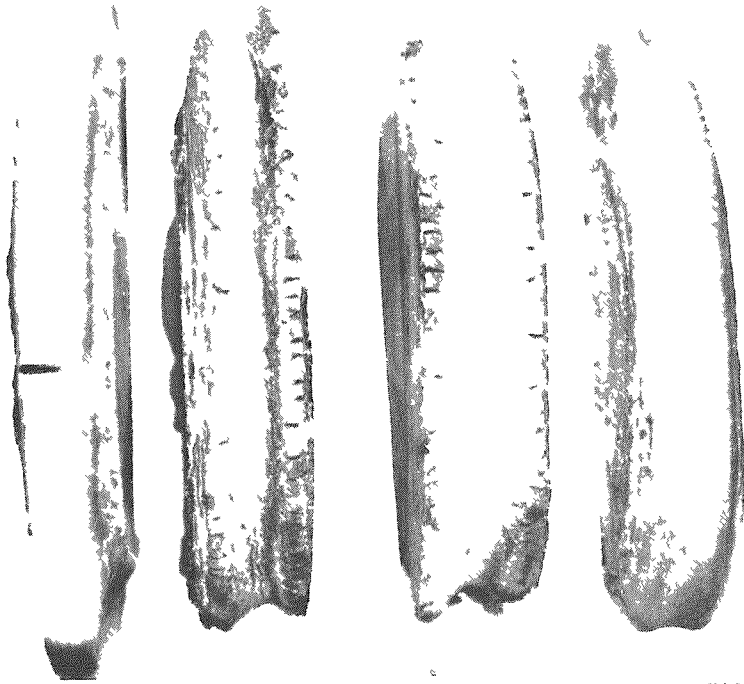
FIGURE 2. EDGE VIEWS OF FORGED (2550 F) SLABS OF NIOBIUM-BASE ALLOYS
