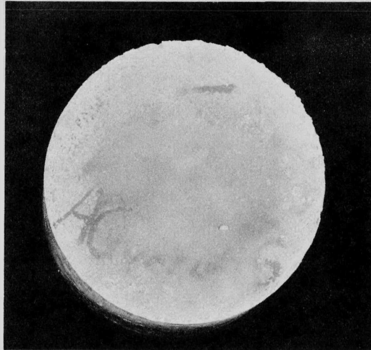
FIGURE 2. FIFTH COMPACT IN A SERIES WHEN LUBRICATING AFTER EVERY SECOND PRESSING WITH AQUADAG
