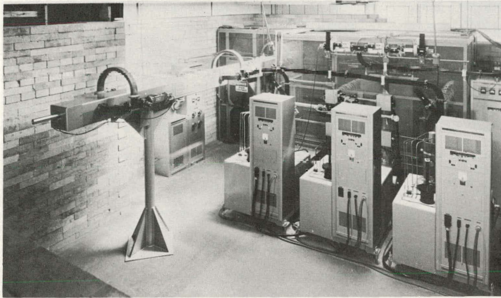
Figure 1. The 5 to 50 MEV electron linear accelerator of the Argonne Cancer Research Hospital. Three klystron stations are shown, one of them a spare. The accelerator tube proper is contained in the protective housing shown on the left side of the picture. (Photograph courtesy of High Voltage Engineering Corporation, Burlington, Massachusetts.)
