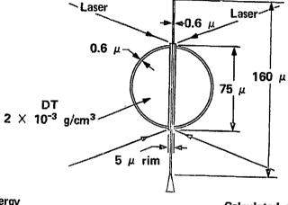
Laser energy East 14 J West 14.6 J Laser puise (~Gaussian) 70 ps Absorbed energy
