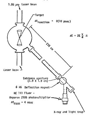
Total flight path = 276.75 cm  $\Rightarrow$   $\Delta E_{FMHM}$  = 130 keV Sensitivity = 5 x 10<sup>-6</sup>  $\alpha$  counts/target reaction TI AND E BEAM VS  $\Delta E_{FWHM}$  OF  $\alpha$
