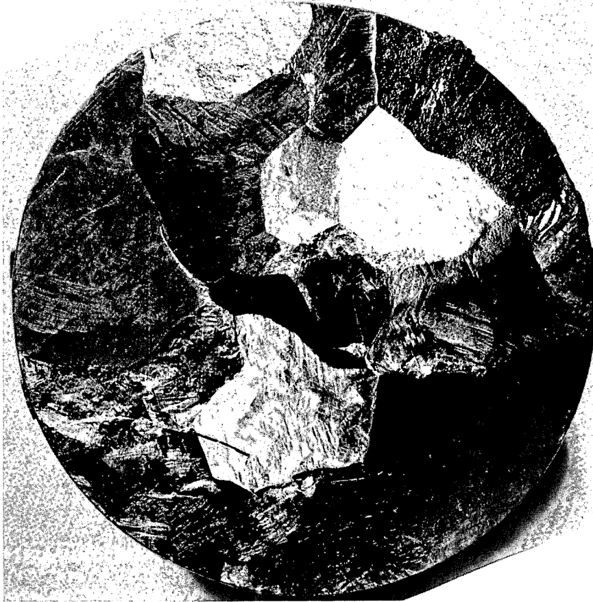
Figure 4. Typical zirconium specimen after vacuum annealing at 1150°C for 48 hours. 7X.
