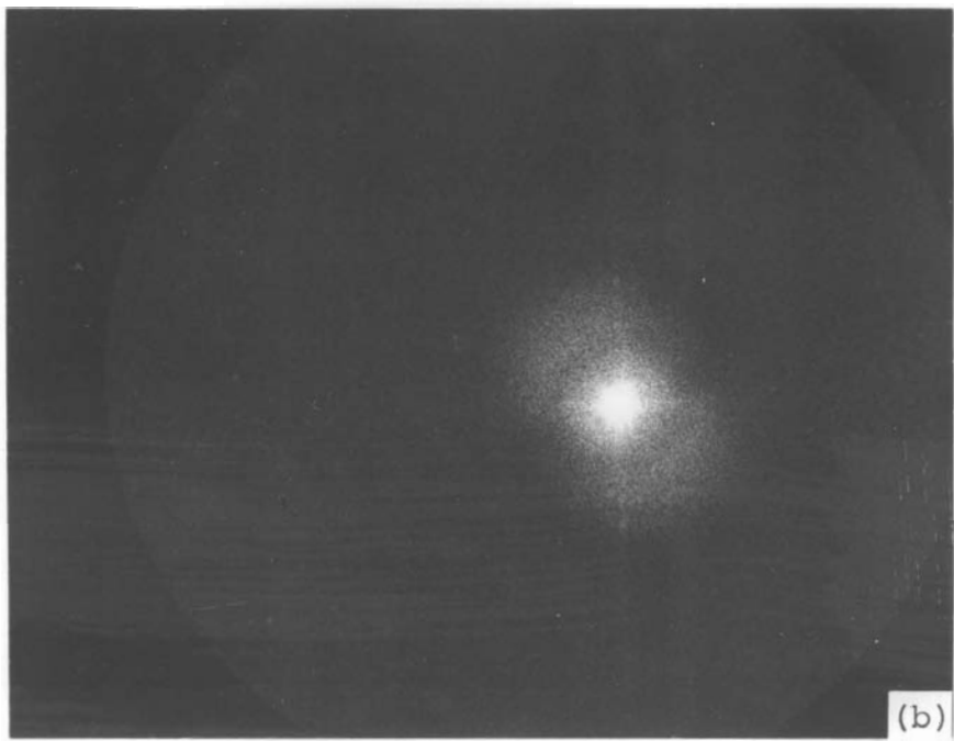
FIGURE 8. FOURIER IMAGE OF FUEL PELLETT AUTORADIOGRAPH
